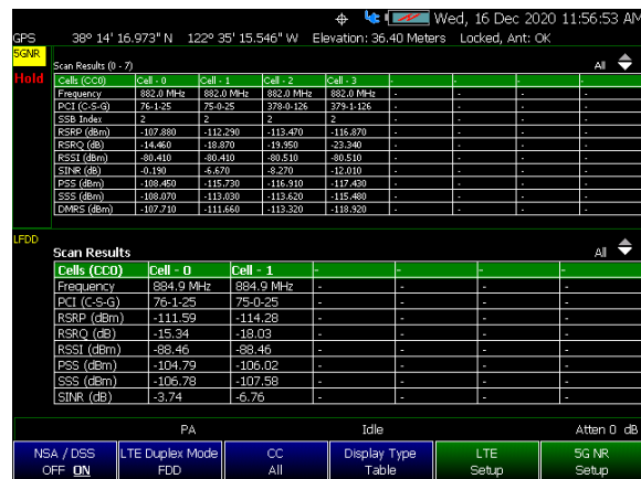
5G DSS on LTE channel
