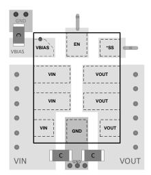
\* SS pin trace must be less than 0.01inch for SS = Float configuration.
