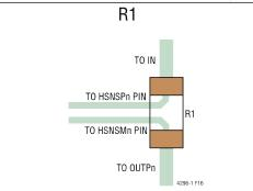
Figure 58. HSNSPn and HSNSMn Pin Kelvin Connection
