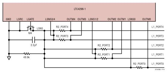
Figure 56. Low-Side Circuit Breaker
