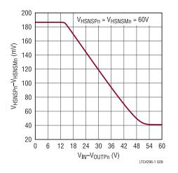
Figure 10. Analog Foldback Current Limit Threshold Voltage vs. VIN-VOUTPN
