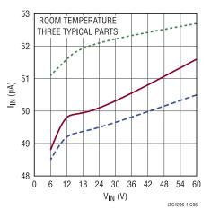
Figure 7. IIN vs. VIN, All Ports in DISABLED State
