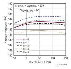
Figure 8. Analog Foldback Current Limit Threshold vs. Temperature
