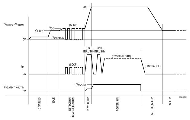
Figure 44. Simplified 802.3cg PSE State Sequence (Not to Scale)
