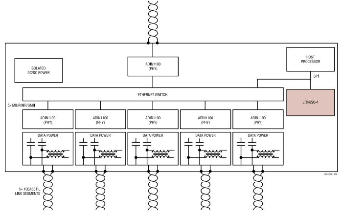
Figure 43. 10BASE-T1L PSE FIELD SWITCH
