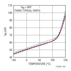
Figure 3. IIN vs. Temperature, All Ports in SLEEP State
