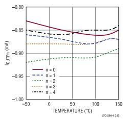
Figure 36. Valid Wakeup Current Low Threshold vs. Temperature
