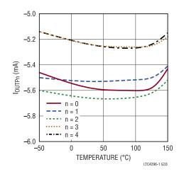
Figure 34. Short-Circuit I<sub>OUTPn</sub> vs. Temperature, SLEEP State
