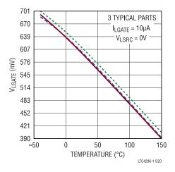
Figure 21. LGATE Pull-Down Voltage vs. Temperature
