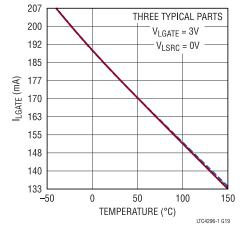
Figure 20. LGATE Pull-Down Current vs. Temperature, LGATE Disabled
