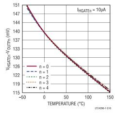
Figure 17. HGATEn Slow Pull-Down Dropout Voltage vs. Temperature
