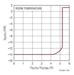
Figure 37. I<sub>VALID</sub> vs. V<sub>OUTPn</sub>-V<sub>OUTMn</sub>
