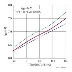
Figure 2. IIN vs. Temperature, All Ports in POWER\_ON State
