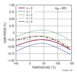
Figure 23. Port ADC Gain Error vs. Temperature
