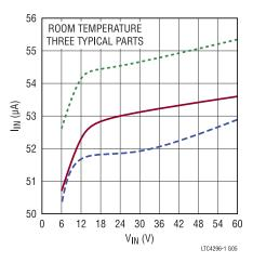
Figure 6. I<sub>IN</sub> vs. V<sub>IN</sub>, All Ports in SLEEP State
