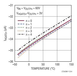
Figure 15. HGATEn Pull-Up Current vs. Temperature
