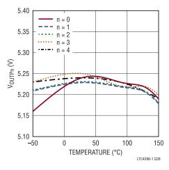
Figure 29. Open-Circuit Detection Voltage vs. Temperature
