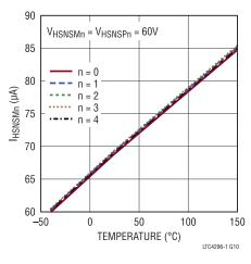
Figure 11. IHSNSMn vs. Temperature, Port in POWER\_ON State
