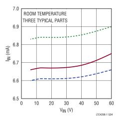
Figure 5. IIN vs. VIN, All Ports in POWER\_ON State
