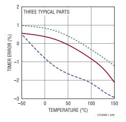
Figure 40. Timer Error vs. Temperature, IDLE, DETECTION/CLASSIFICATION, or POWER\_ON States
