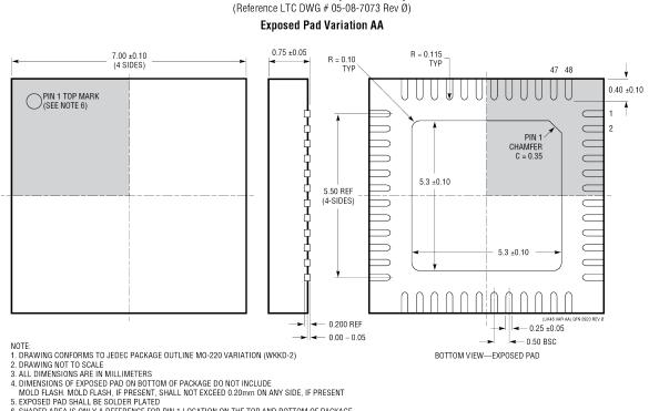
$\begin{array}{c} \text{UK Package} \\ \text{48-Lead Plastic QFN (7mm <math display="inline">\times$  7mm)} \end{array}
