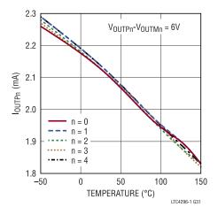
Figure 32. IDISCHARGE vs. Temperature
