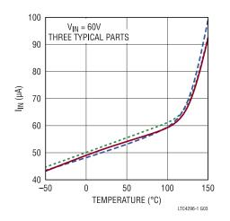
Figure 4. I<sub>IN</sub> vs. Temperature, All Ports in DISABLED State
