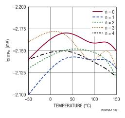
Figure 35. Valid Wakeup Current High Threshold vs. Temperature
