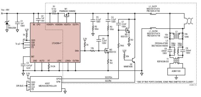
Figure 60. High-Current, Low-Droop Application Circuit
