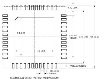
APPLY SOLDER MASK TO AREAS THAT ARE NOT SOLDERED
