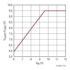
Figure 19. Low-Side N-Channel GATE Drive vs. V<sub>IN</sub>
