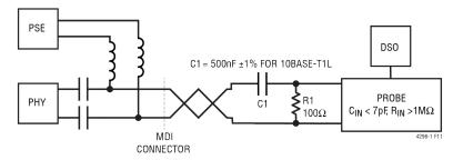
Figure 53. Power Supply Ripple Measurement Setup
