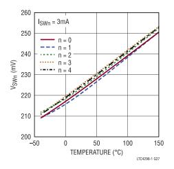
Figure 28. SWn Low Output Voltage vs. Temperature
