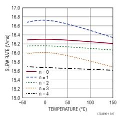
Figure 18. HGATEn Inrush Slew Rate vs. Temperature
