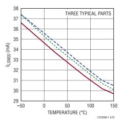
Figure 13. Deep Sleep Return Path Forward Fault Threshold vs. Temperature
