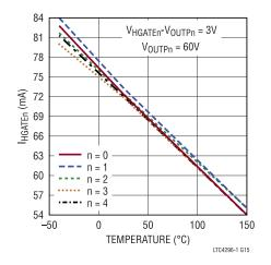
Figure 16. HGATEn Fast Pull-Down Current vs. Temperature
