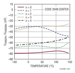
Figure 24. Port ADC Offset vs. Temperature
