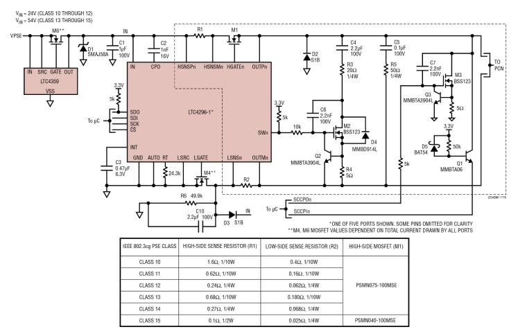
Figure 57. LTC4296-1 PSE Port with MDI Fault Tolerance
