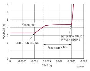
Figure 45. Typical Valid Detection Sequence Waveform
