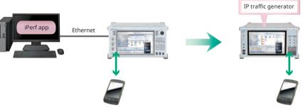
For the transmission and reception of the UE, use iPerf application which is widely used for throughput testing.
