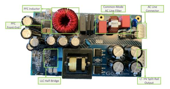
Figure 3 Gen2 GaN Switched-Mode Power Supply Evaluation Board GS-EVB-AUD-SMPS2-GS
