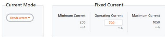
Figure 5: Setting of the operating current
