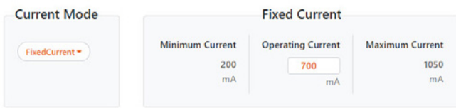
Figure 5: Setting of the operating current
