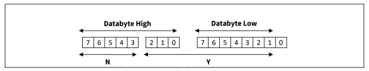
Figure 24 11-Bit Linear Data Format
