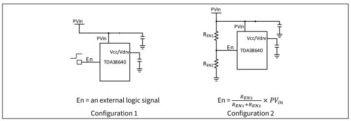
Figure 17 Enable Configurations
