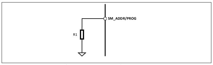
Figure 22 SM-ADDR/PROG Pin Components
