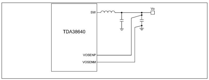
Figure 18 Output voltage sensing connections
