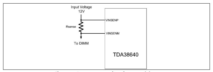
Figure 19 Input current sensing using external shunt
