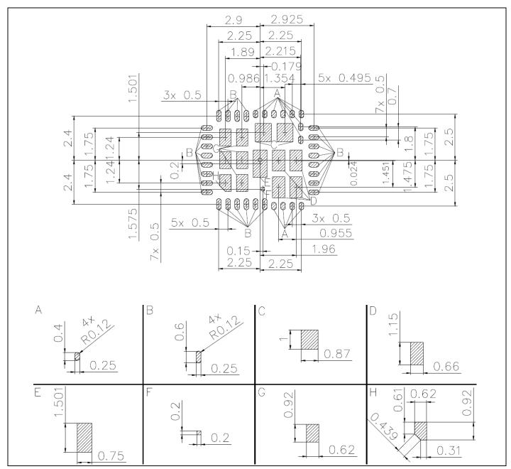
Figure 28 Stencil pad size and spacing (all dimensions in mm)
