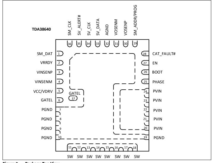
Figure 2 Package Top View
