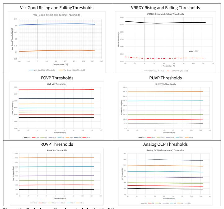
Figure 12 Typical operating characteristics (set 2 of 2)
