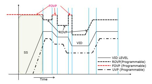
Figure 21 OVP example diagram. Note the situations in which FOVP takes over from ROVP.
