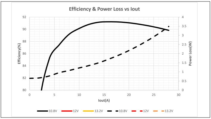
Figure 8 Typical efficiency and power loss curves, PV<sub>in</sub> = Varying, F<sub>sw</sub> = 1000 kHz
