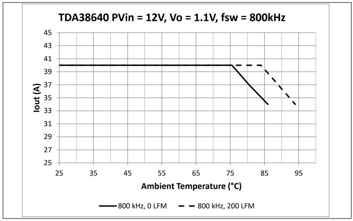
Figure 9 Thermal de-rating curves, PV<sub>in</sub> = 12 V, V<sub>out</sub>=1.1 V, f<sub>sw</sub> = 800 kHz, VCC = Internal LDO
