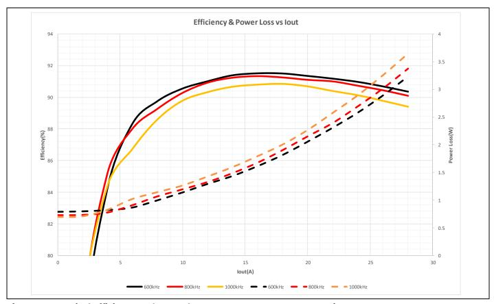
Figure 6 Typical efficiency and power loss curves, PV<sub>in</sub> = 12 V, F<sub>sw</sub> = Varying
