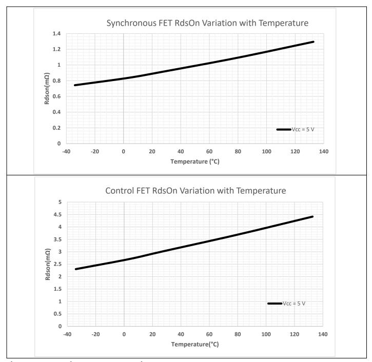
Figure 10 R<sub>DS(on)</sub> of MOSFETs over Junction Temperature
