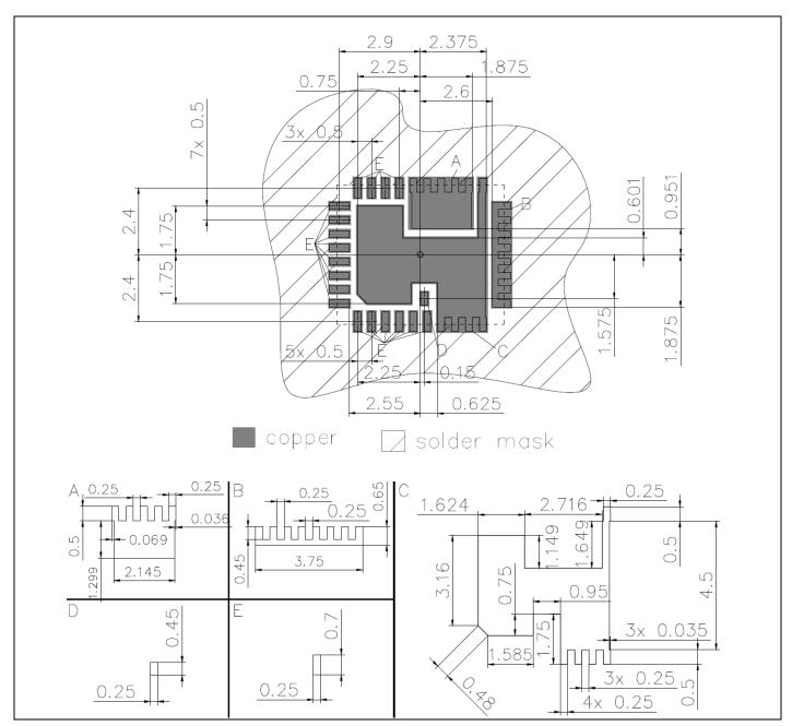
Figure 27 Solder resist
