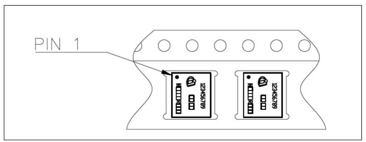
Figure 33 Pin 1 orientation in the Tape & reel
