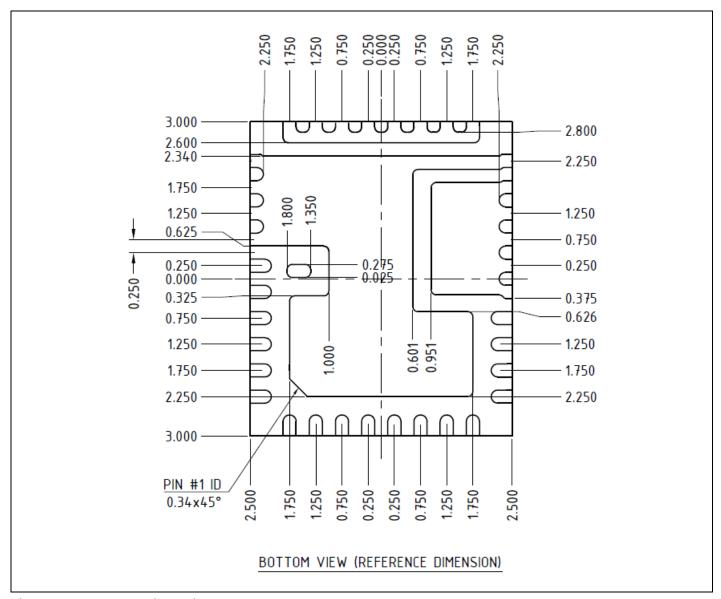
Figure 32 Package Dimensions- Pad Layout
