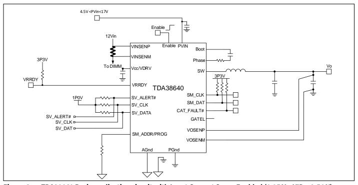
Figure 4 TDA38640 Basic application circuit with Input Current Sense Enabled (0.25 V ≤ VID ≤ 2.56 V)
