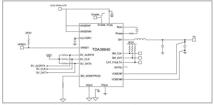
Figure 5 TDA38640 Application Circuit with Input Current Sense Disabled (0.25 V ≤ VID ≤ 2.56 V)
