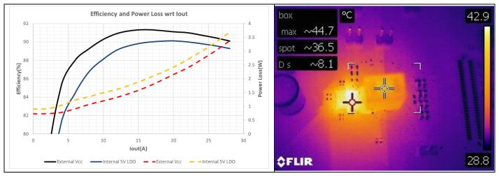
Figure 7 Typical efficiency & power loss curve plus thermal image at full load of 28 A with Internal LDO,  $PV_{in}$  = 12 V,  $F_{sw}$  = 800 kHz
