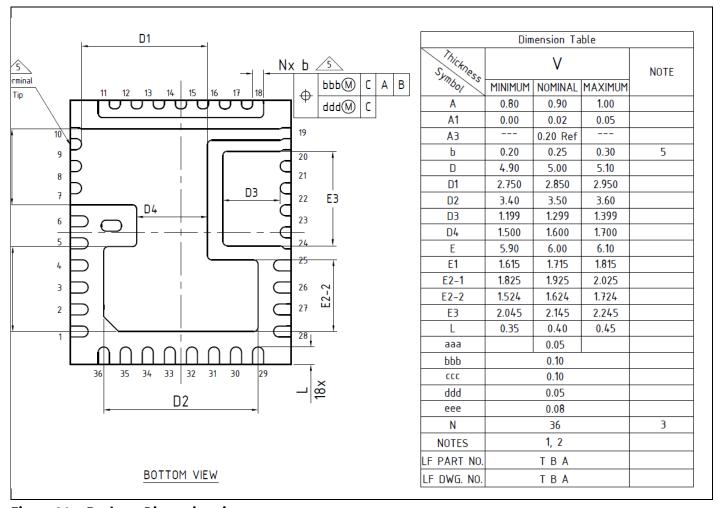
Figure 31 Package Dimensions in mm
