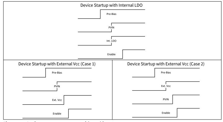
Figure 15 Device power-on sequence with pre-bias.
