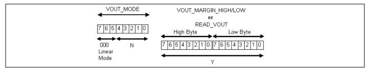
Figure 25 16-BIT Linear Data Format
