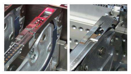
Figure 16. A representative of a LUXEON LED emitter that is held by a magnet strip (left). LUXEON Rubix is attracted to magnets. Example of Panasonic CM402 feeder with magnet strip installed (right).
