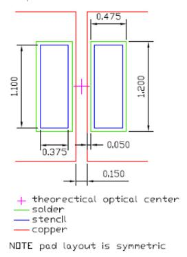
Figure 5. Recommended footprint layout for LUXEON Rubix. All dimensions are in millimeters.
