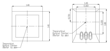
Figure 2. The theoretical optical centers of LUXEON Rubix. All dimensions are in millimeters.
