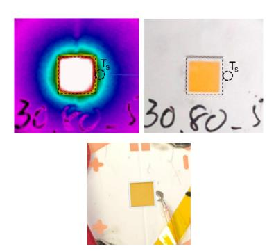
Figure 25: The  $T_s$  location is defined next to a representative two-pad LED package outline. Top left shows the result of thermal imaging camera showing the temperature profile of the top surface of the Al-MCPCB. Top right shows the defined  $T_s$  location.
