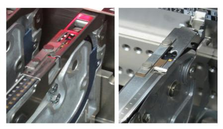
Figure 15. Samsung SM421 (left) and Juki KE-2080L (right) feeders.
