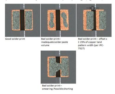
Figure 10. Examples of good and bad solder print.
