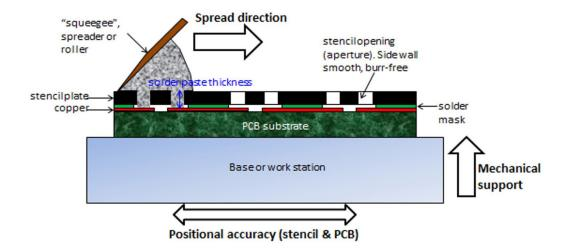
Figure 9. Stencil printing process.
