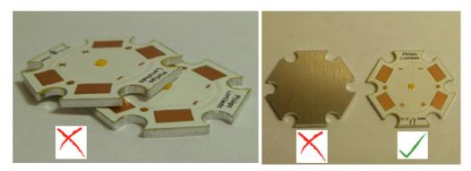
Figure 4. Do not stack assembled LED on PCBs on top of each other (left). Do not place assembled PCBs with the top side down on any surface (right).
