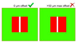
Figure 8. A maximum of 50µm mis-registration between solder mask (green) and copper pattern (red) is preferred.
