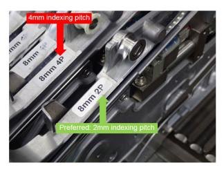
Figure 17. An example of Samsung SM421 feeder with 2mm and 4mm indexing pitches.
