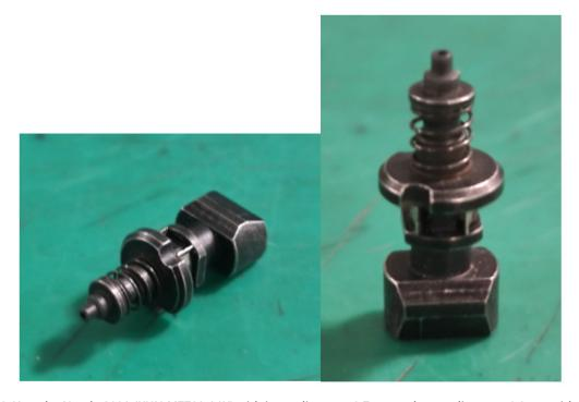
Figure 20: Yamaha Nozzle 309A (KHN-M7790-A1X) with inner diameter 0.7mm and outer diameter 1.2mm with Teflon tip.
