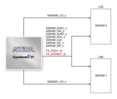
Figure 3-25 Connections between FPGA and SSRAM
