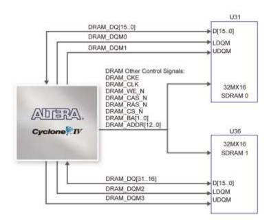
Figure 3-26 Connections between FPGA and SDRAM
