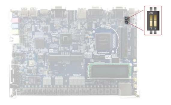
Figure 3-1 The Power Up Sequence Control Switch
