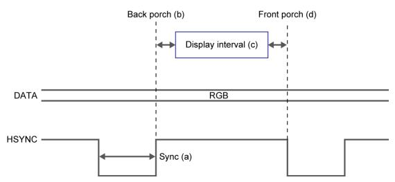
Figure 3-18 VGA horizontal timing specification
