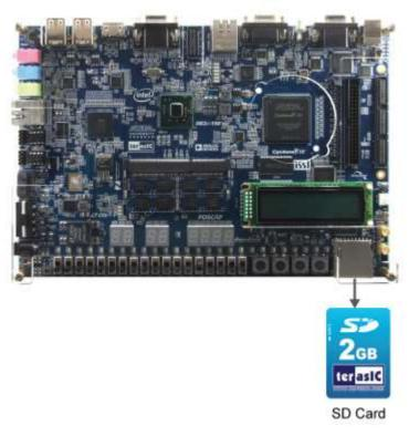
Figure 5-5 Insert SD Card for the SD Card Demonstration
