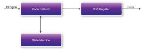
Figure 5-9 The IR Receiver controller
