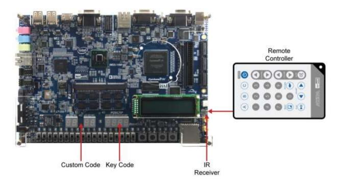
Figure 5-11 The Setup of the IR receiver demonstration
