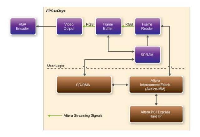
Figure 6-7 Block diagram of the PCI Express design in FPGA
