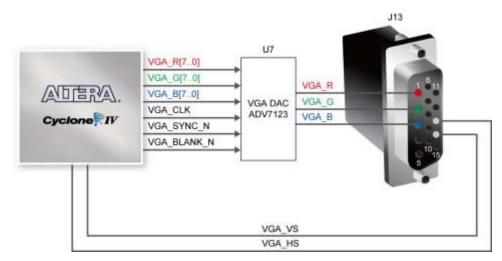
Figure 3-17 Connections between FPGA and VGA
