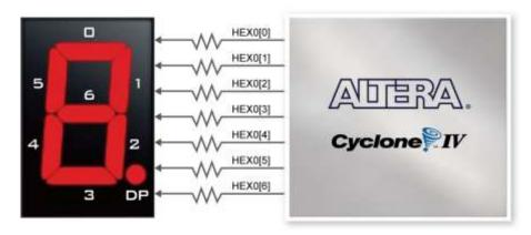
Figure 3-11 Connections between the 7-segment display HEX0 and Cyclone IV GX FPGA
