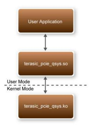
Figure 6-3 PCI Express Software Stack on Yocto
