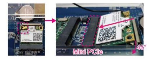
6. Push down the WiFi module into the slot.
