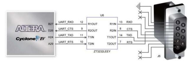
Figure 3-19 Connections between FPGA and ZT3232 (RS-232) chip
