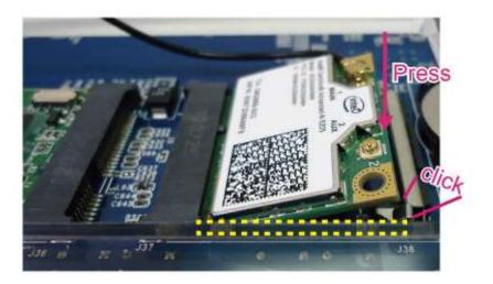
7. Confirm the sections circled are secured.
