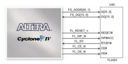
Figure 3-27 Connections between FPGA and Flash
