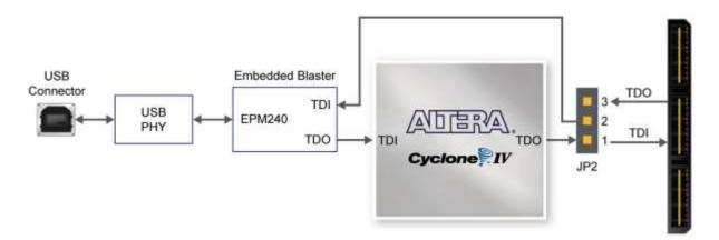
Figure 3-2 The JTAG chain on DE2i-150 board
