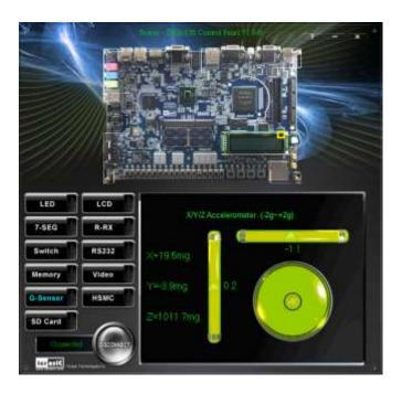
Figure 2-13 Testing the G-sensor
