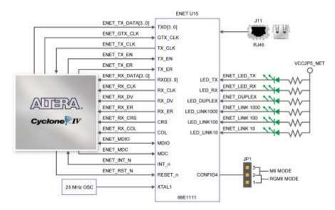
Figure 3-20 Connections between FPGA and Ethernet
