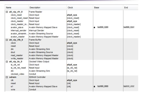
Figure 6-8 User Logic components in Altera Qsys
