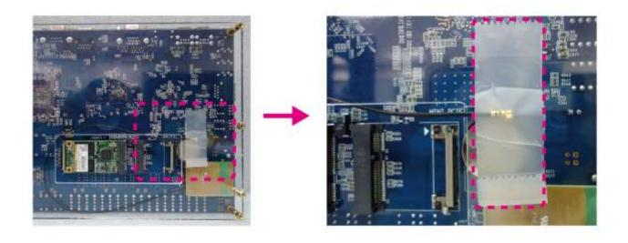
4. Connect the other end of antenna (A) to the WiFi module (B) and press the conjunction to make sure it's secured.
