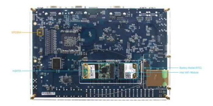
Figure 1-2 The DE2i-150 board (bottom view)
