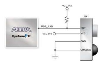
Figure 3-24 Connection between FPGA and IR
