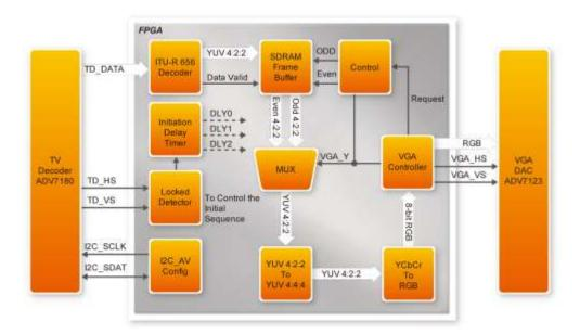
Figure 5-1 Block diagram of the TV box demonstration
