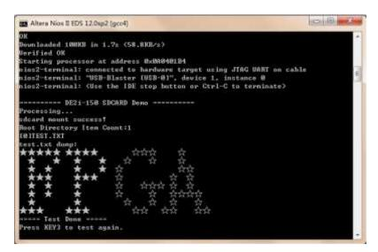
Figure 5-6 Running results of the SD Card demonstration
