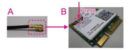
5. Install the WiFi module to the mini PCIe connector on DE2i-150. Bend the cable circled before installing the WiFi module to keep the cable connected.
