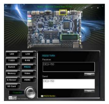
Figure 2-9 RS-232 Serial Communication
