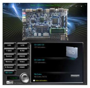
Figure 2-8 Reading the SD Card Identification and Specification
