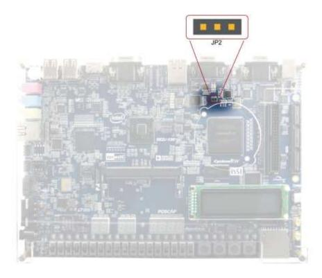
Figure 3-3 The JTAG chain configuration header
