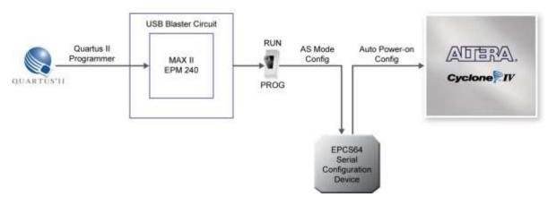
Figure 3-6 The AS configuration scheme
