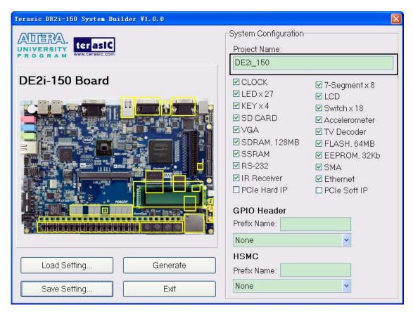
Figure 4-3 The DE2i-150 Board Type and Project Name
