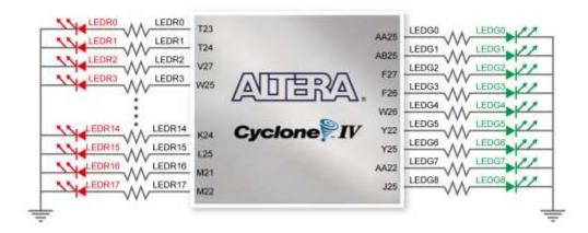
Figure 3-10 Connections between the LEDs and Cyclone IV GX FPGA
