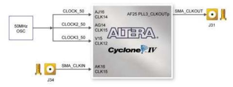
Figure 3-12 Block diagram of the clock distribution
