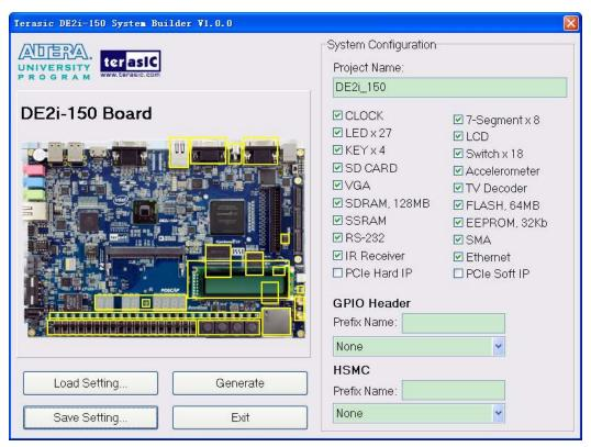
Figure 4-2 The DE2i-150 System Builder window
