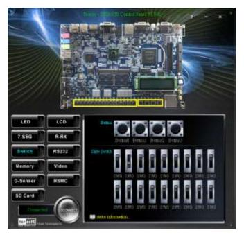
Figure 2-6 Monitoring switches and buttons
