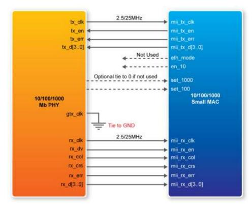
Figure 5-16 PHY connected to the MAC via MII
