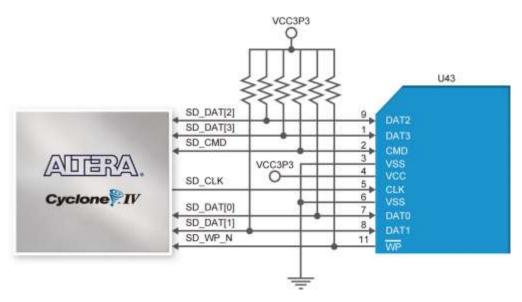
Figure 3-28 Connections between FPGA and SD Card Socket
