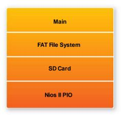
Figure 5-4 Software Stack of the SD Card Demonstration
