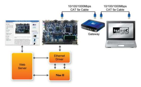
Figure 5-19 System Principle Diagram
