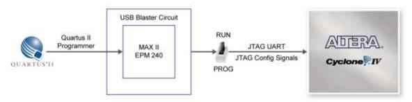
Figure 3-4 The JTAG configuration scheme
