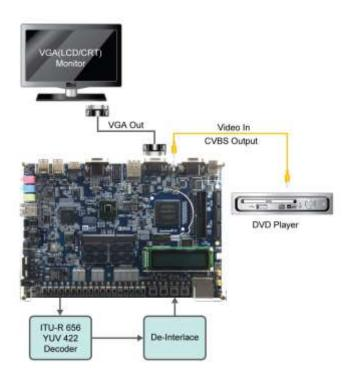
Figure 5-2 The setup for the TV box demonstration
