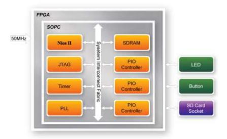
Figure 5-3 Block Diagram of the SD Card Demonstration
