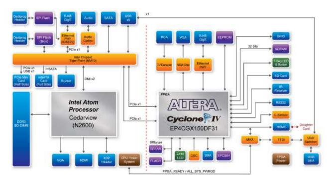
Figure 1-3 Block Diagram of DE2i-150
