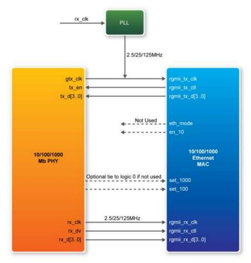
Figure 5-17 PHY connected to the MAC via RGMII
