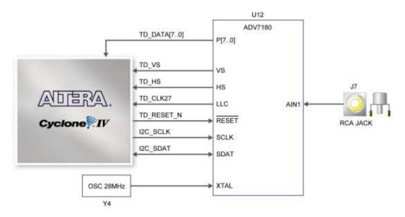
Figure 3-22 Connections between FPGA and TV Decoder
