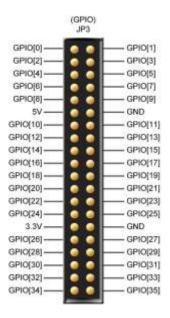
Figure 3-15 GPIO Pin Arrangement
