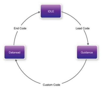
Figure 5-10 State shift diagram of State Machine
