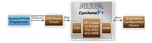
Figure 3-10 Programming a quad serial configuration device with SFL solution
