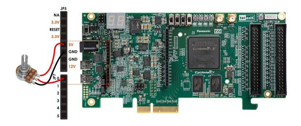
Figure 5-20 ADC Reading Demo hardware setup
