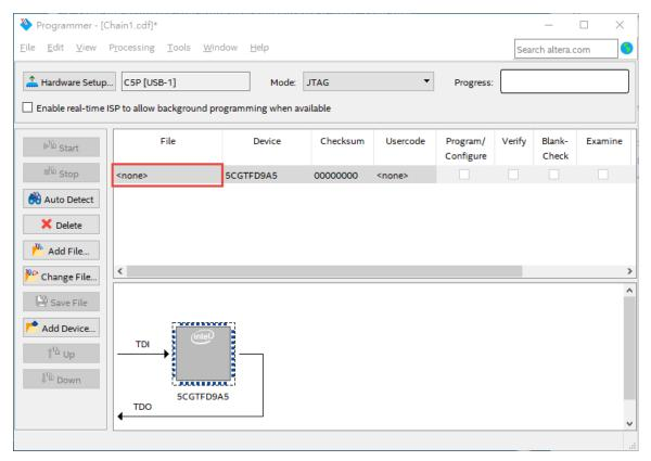
Figure 6-7 Quartus Prime Programmer detectes the FPGA device
