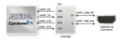
Figure 3-20 Connections between the FPGA, CP2102N chip and USB Mini-B
