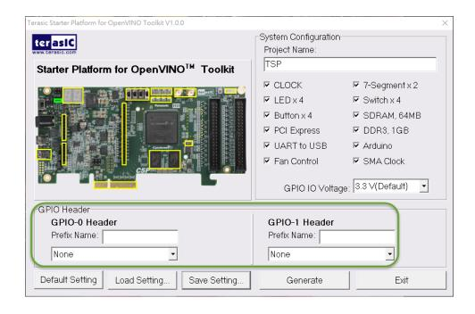
Figure 4-5 GPIO Expansion
