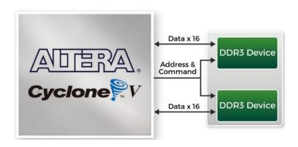
Figure 3-19 Connections between FPGA and DDR3
