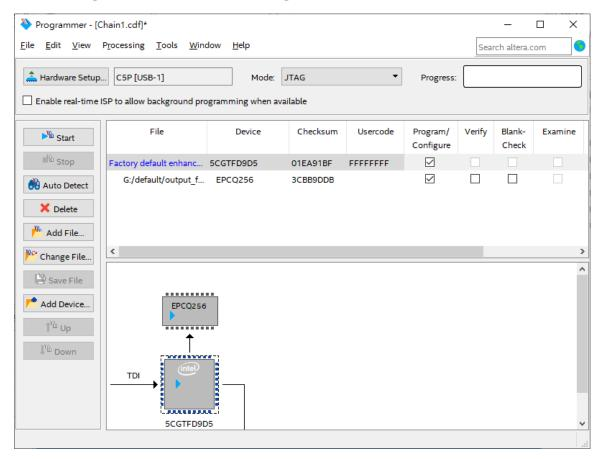
Figure 6-8 Quartus Prime Programmer window with .jic file
