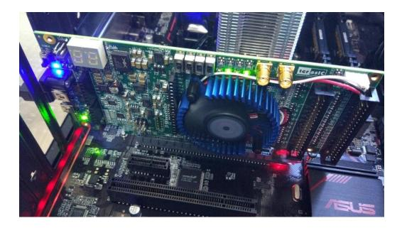
Figure 7-3 Install the FPGA board on the PC
