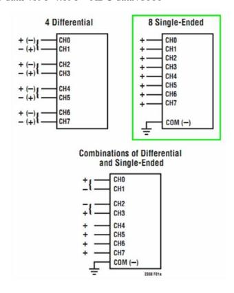
Figure 5-19 Example MUX Configurations
