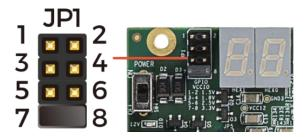
Figure 3-24 Short pin 7 and pin 8 of JP1
