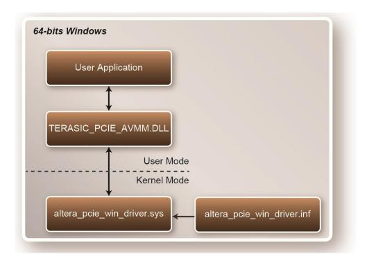
Figure 7-2 PCI Express Software Stack
