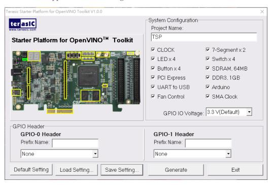
Figure 4-2 Starter Platform for OpenVINOTM ToolkitSystem Builder window
