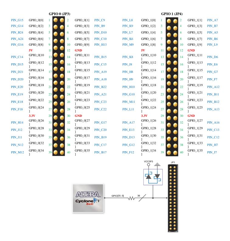
Figure 3-25 Connections between the GPIO connector and Cyclone V FPGA
