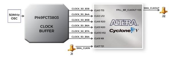
Figure 3-12 Block diagram of the clock distribution on Starter Platform for OpenVINO<sup>TM</sup> Toolkit
