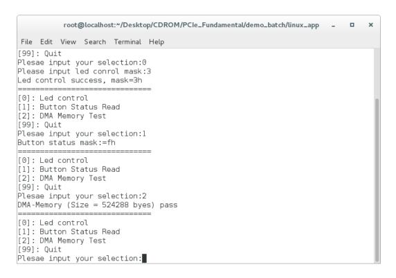
Figure 8-8 Screenshot of DMA Memory Test Result
