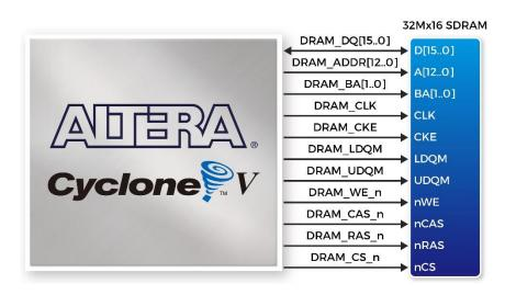
Figure 3-18 Connections between the FPGA and SDRAM
