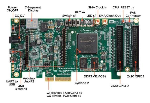
Figure 2-1 Starter Platform for OpenVINO<sup>TM</sup> Toolkit (top view)
