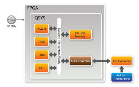
Figure 5-17 ADC System Block Diagram
