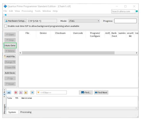
Figure 3-2 Detect FPGA device in JTAG mode
