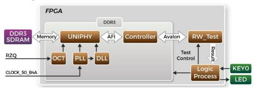
Figure 5-5 Block Diagram of DDR3 Demostration
