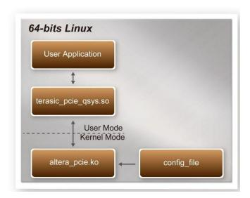
**Figure 8-2 PCI Express Software Stack**
