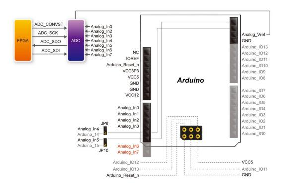
Figure 3-22 Connection and pin assignments of Arduino analog input (ADC)
