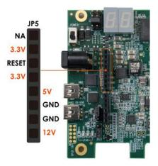
Figure 5-16 Power supply from Starter Platform for OpenVINO<sup>TM</sup> Toolkit
