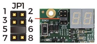
Figure 3-23 Short pin5 and pin 6 of JP1
