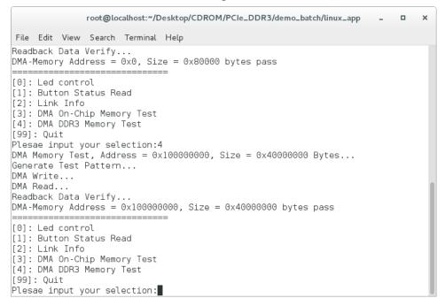
Figure 8-14 Screenshot of DDR3 Memory DAM Test Result
