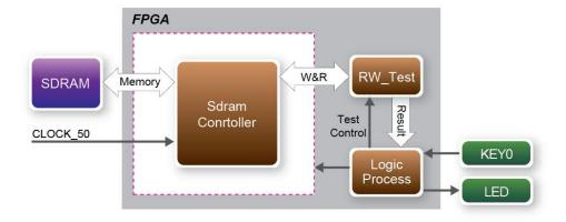
Figure 5-4 Block Diagram of Verilog SDRAM Test
