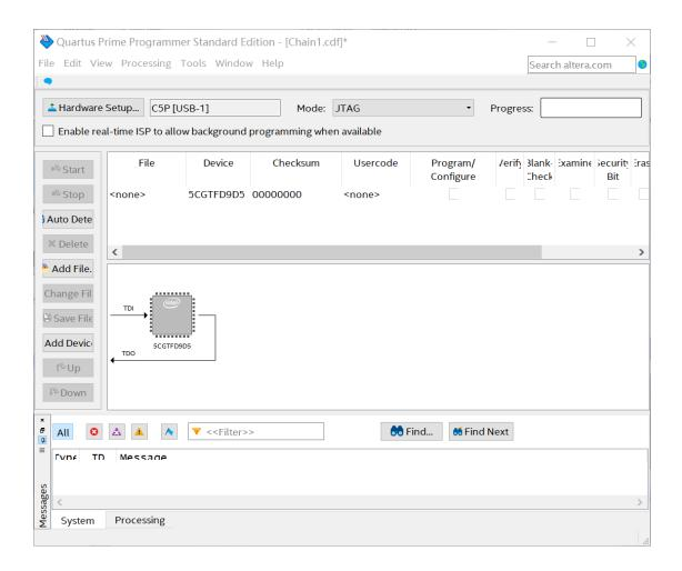
Figure 3-5 FPGA detected in Quartus programmer
