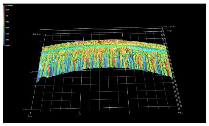
Fig. 6 Surface topography of the semi-crystalline sample. Blue indicates height lower than CAD and red indicates height higher than CAD.
