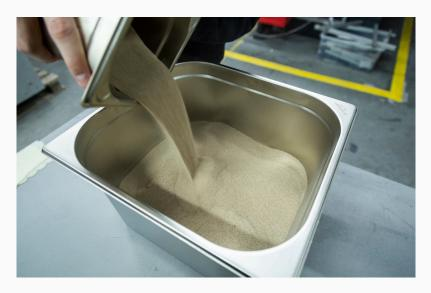
After the printing is done and the printing chamber has cooled down to room temperature, the models need to be removed from the build plate and placed in a metal container filled to roughly 10 mm height with quartz sand with a grain gradation of approximately 0.6 mm.
