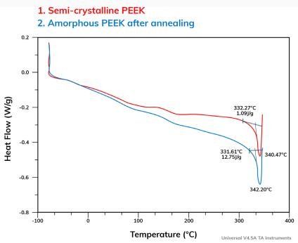
Fig. 1 DSC curves from heating cycles of semi-crystalline PEEK samples and amorphous PEEK samples annealed to achieve semi-crystalline phase.
