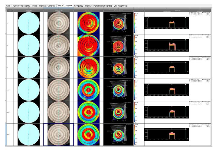
Fig. 4 Three semi-crystalline samples at the top and three amorphous samples at the bottom. Red color indicates higher dimensional deviation from the CAD model.
