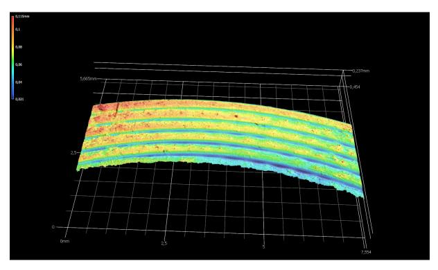
Fig. 7 Surface topography of the amorphous sample. Blue indicates height lower than CAD and red indicates height higher than CAD.
