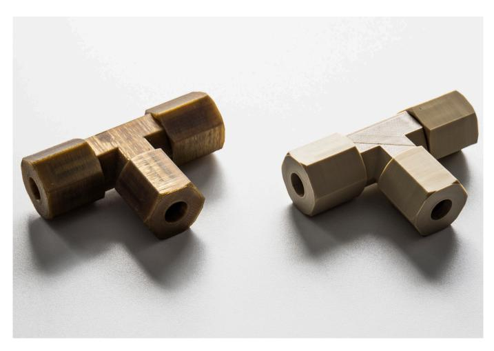
Fig. 3 Amorphous samples with accurate geometry on the left, semi-crystalline samples with visible imperfections on the right.
