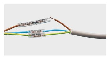
Set the connector and pull back the shrink tube.
