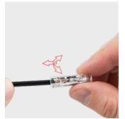
Removal: For solid conductors, twist alternately left and right while pulling the connector. For stranded conductors, cut the wire and use a new connector.
