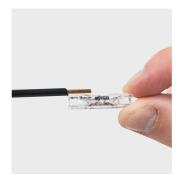
Strip conductor to 10 mm.
