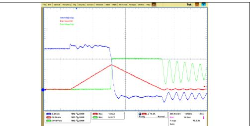
FIGURE 2-43: High-Voltage Auxiliary E-Fuse Variant A Short-Circuit. Measurement.
