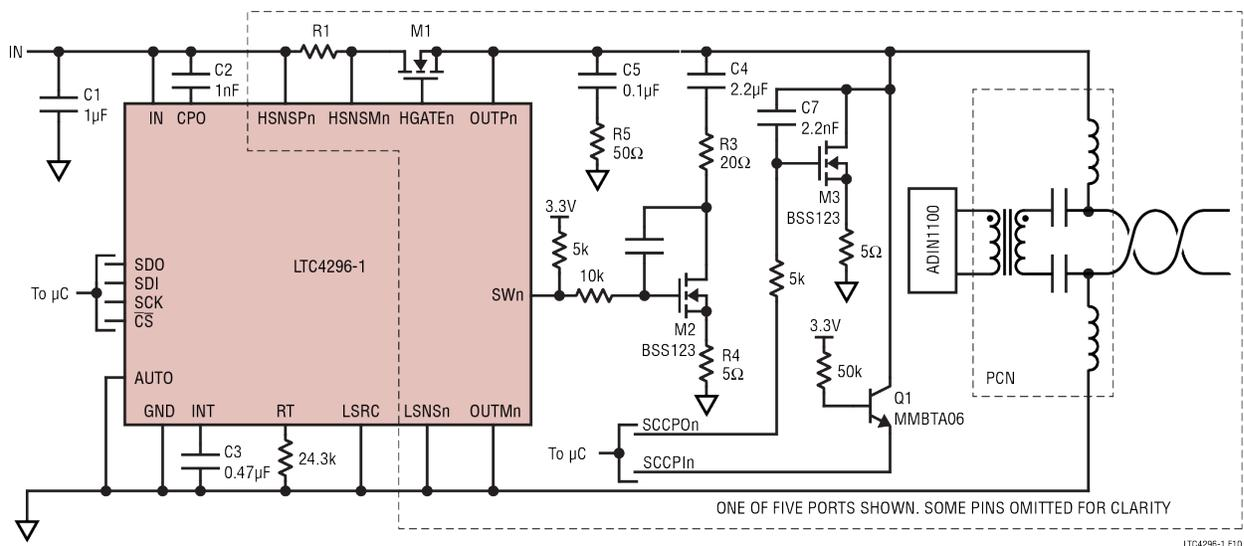
Figure 52. Typical LTC4296-1 Circuit (1 of 5 ports Shown)
