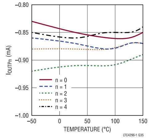
Figure 36. Valid Wakeup Current Low Threshold vs. Temperature
