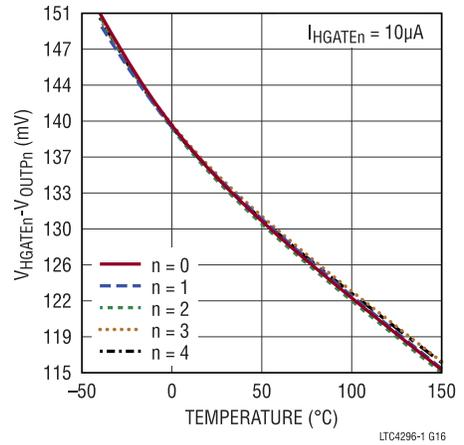
Figure 17. HGATEn Slow Pull-Down Dropout Voltage vs. Temperature
