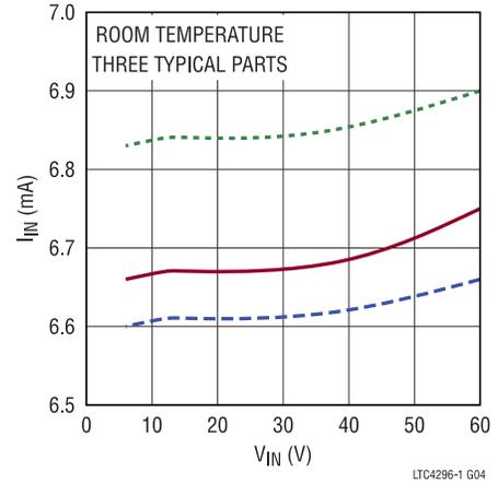
Figure 5.  $I_{IN}$  vs.  $V_{IN}$ , All Ports in POWER\_ON State
