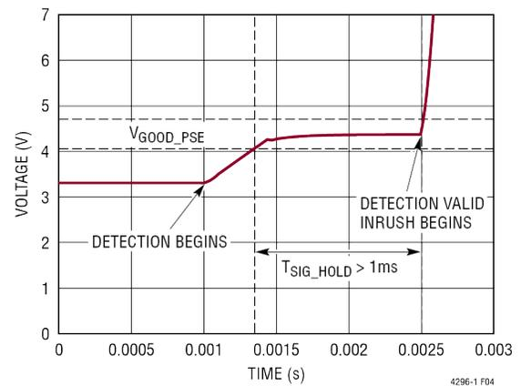
Figure 45. Typical Valid Detection Sequence Waveform
