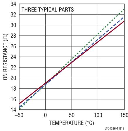
Figure 14. Deep Sleep Return Path On Resistance vs. Temperature
