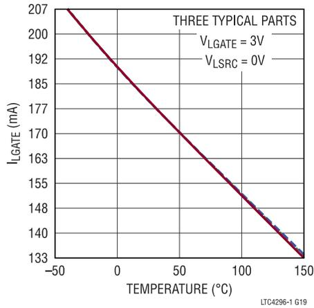
Figure 20. LGATE Pull-Down Current vs. Temperature, LGATE Disabled
