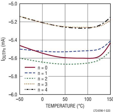
Figure 34. Short-Circuit  $I_{OUTPn}$  vs. Temperature, SLEEP State
