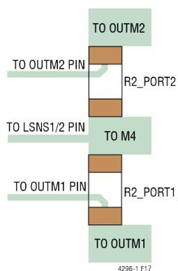
Figure 59. Shared LSNS1/2, OUTM1 and OUTM2 Pins Example Kelvin Sense Layout
