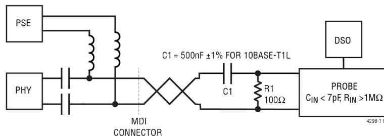
Figure 53. Power Supply Ripple Measurement Setup
