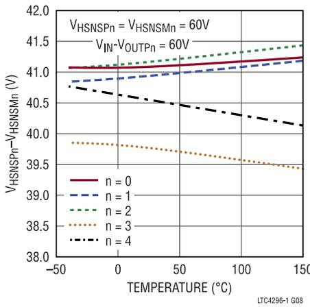
Figure 9. Analog Foldback Current Limit Threshold vs. Temperature
