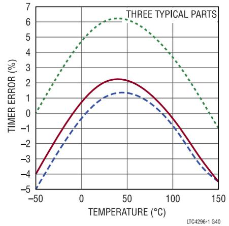
Figure 41. Timer Error vs. Temperature, All Ports *DISABLED*, or *SLEEP* States
