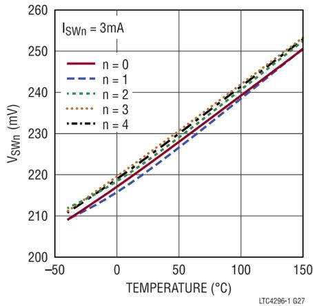
Figure 28. SWn Low Output Voltage vs. Temperature
