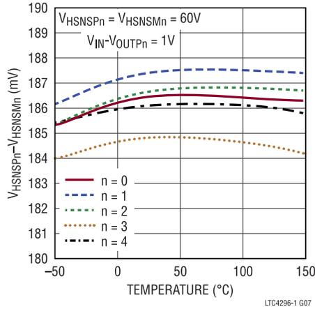
Figure 8. Analog Foldback Current Limit Threshold vs. Temperature
