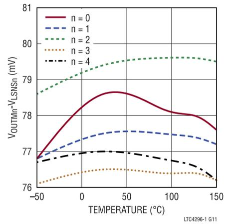
Figure 12. LGATE Circuit Breaker Threshold vs. Temperature
