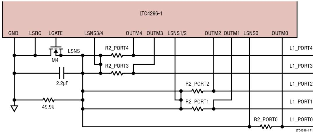
Figure 56. Low-Side Circuit Breaker
