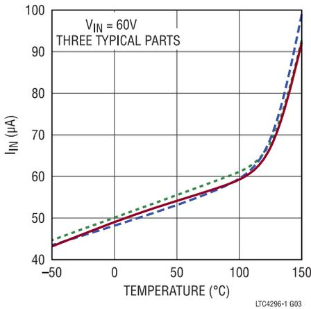
Figure 4.  $I_{IN}$  vs. Temperature, All Ports in DISABLED State
