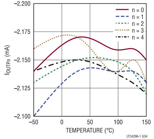
Figure 35. Valid Wakeup Current High Threshold vs. Temperature
