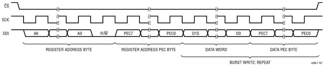
Figure 49. SPI Write
