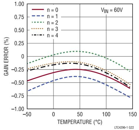
Figure 23. Port ADC Gain Error vs. Temperature
