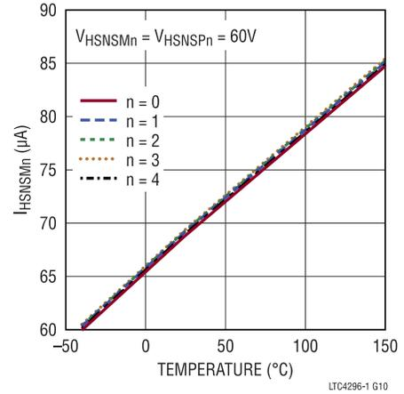
Figure 11.  $I_{HSNSMn}$  vs. Temperature, Port in POWER\_ON State
