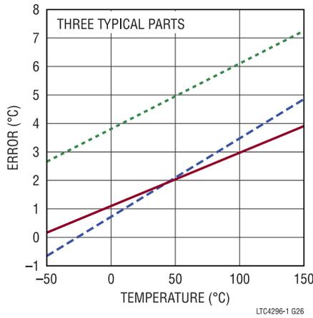
Figure 27. Internal Temperature Sensor Error vs. Temperature
