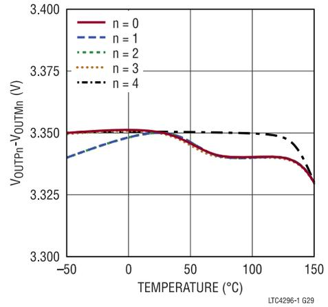
Figure 30. SLEEP State Open-Circuit Output Voltage vs. Temperature
