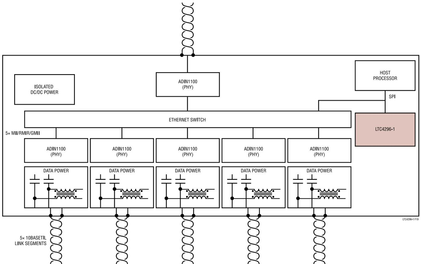
**Figure 43. 10BASE-T1L PSE FIELD SWITCH**
