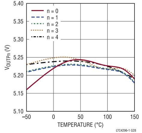
Figure 29. Open-Circuit Detection Voltage vs. Temperature
