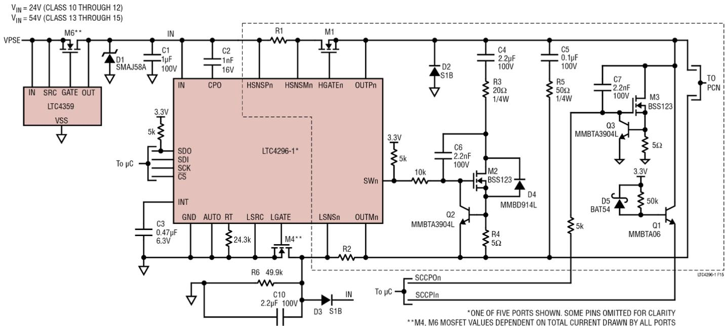
Figure 57. LTC4296-1 PSE Port with MDI Fault Tolerance
