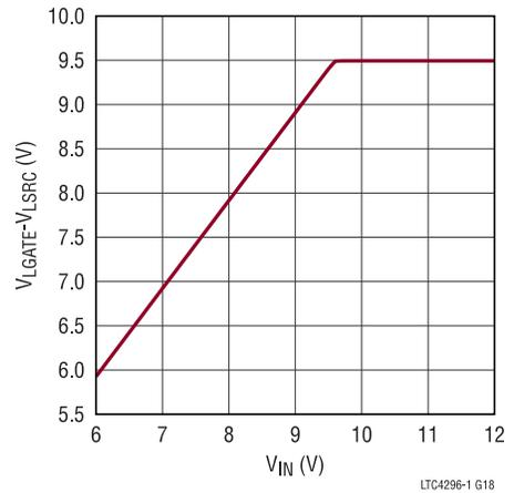
Figure 19. Low-Side N-Channel GATE Drive vs. VIN
