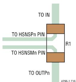
Figure 58. HSNSPn and HSNSMn Pin Kelvin Connection
