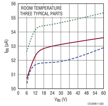
Figure 6.  $I_{IN}$  vs.  $V_{IN}$ , All Ports in SLEEP State
