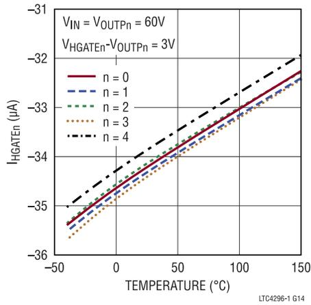
Figure 15. HGATEn Pull-Up Current vs. Temperature
