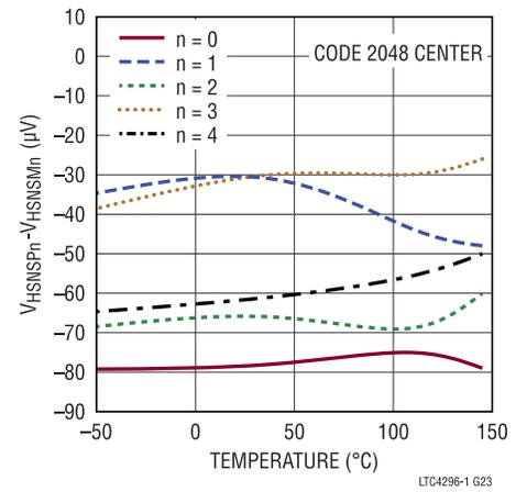
Figure 24. Port ADC Offset vs. Temperature
