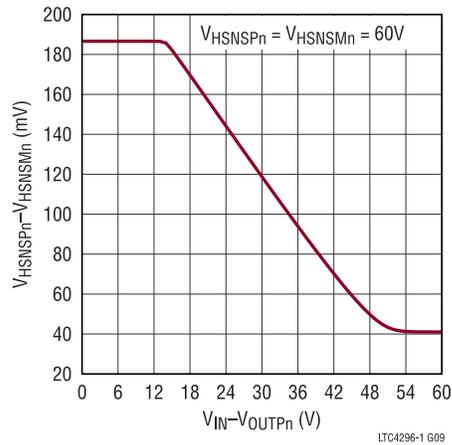
Figure 10. Analog Foldback Current Limit Threshold Voltage vs.  $V_{IN} - V_{OUTn}$
