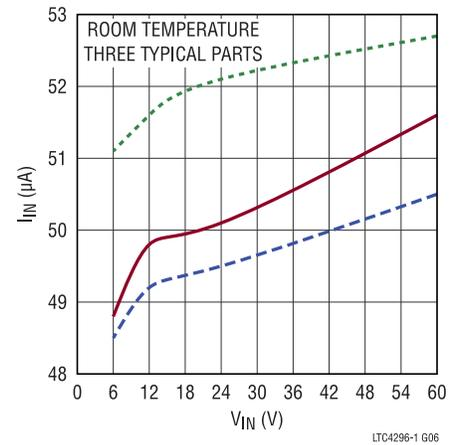
Figure 7.  $I_{IN}$  vs.  $V_{IN}$ , All Ports in DISABLED State
