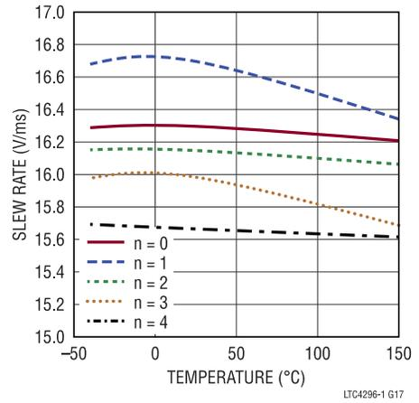
Figure 18. HGATEn Inrush Slew Rate vs. Temperature
