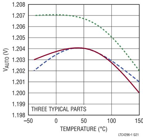
Figure 22. AUTO Input Threshold Voltage vs. Temperature, Rising-Edge
