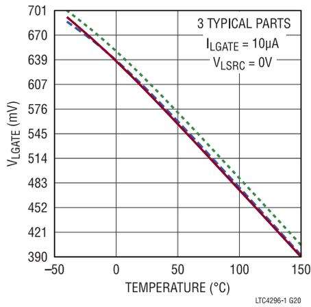
Figure 21. LGATE Pull-Down Voltage vs. Temperature
