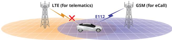
One-touch handover test settings save time and eliminate user worries. The following cells are supported.
