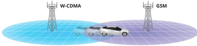
Figure shows the situation when the IVS switches from a 4G network connection used by Telematics services during driving to a 2G/3G network connection for eCall functions when an accident occurs. To emulate this type of test environment, the MD8475B and eCall Tester software perform the handover and CS Fallback switching tests in combination with the eCall function test.
