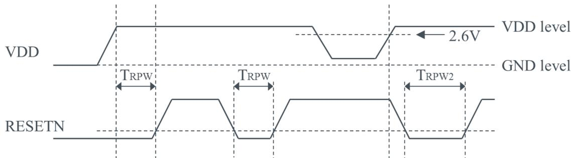
(\*1) Input High level signal, following an assert duration (longer than TRPW), to RESETN after VDD completely rising for start-up.
