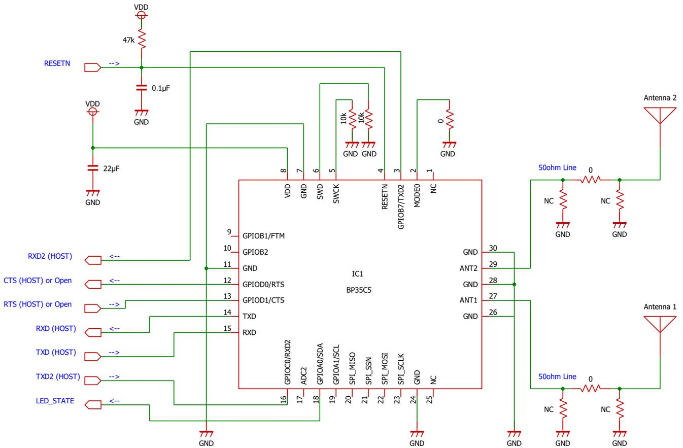
Fig. 2.2. Reference Peripheral Circuit Diagrams
