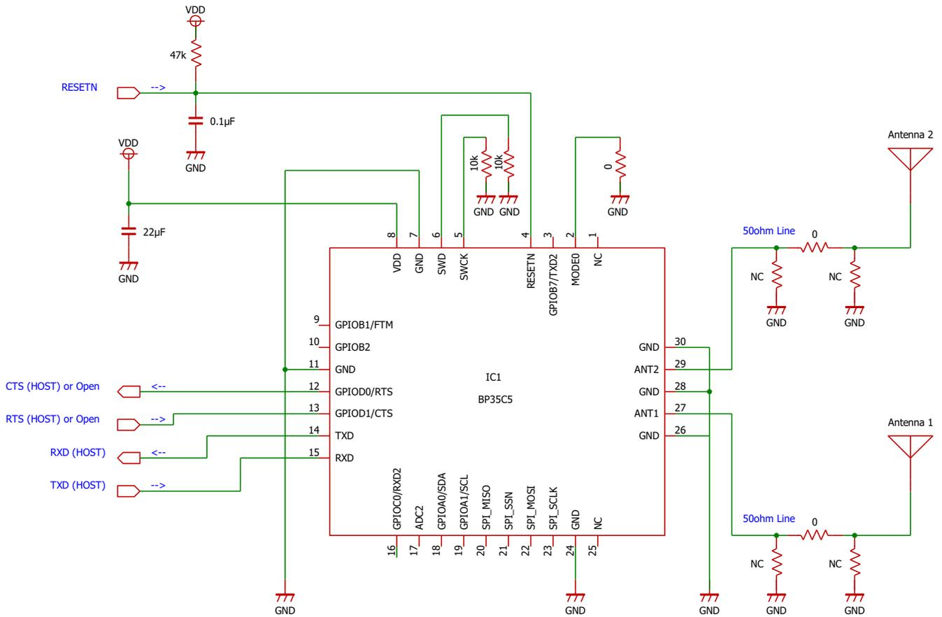
Fig. 2.1. Reference Peripheral Circuit Diagrams
