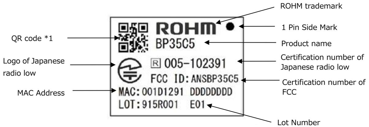
Fig. 4. Marking Specification
