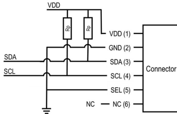
The sensor needs to be supplied with 5 V +/- 10%. Constant supply values are desired for optimal performance. When the sensor is in measurement mode (after first 60 seconds) the typical average supply current is 63mA, while 70 mA at maximum. Considering the start, and the other operation modes, the maximum peak current is 110 mA. The operation of the sensor follows the flowchart:
