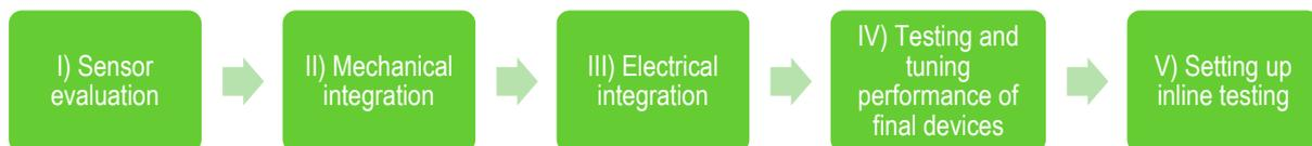
Please note that some process steps will need iterations. Typically, after the first testing of the final device performance, adjustments of the mechanical and electrical integration still need to be done to optimize performance and tune the design for the desired behavior. The following sections will guide you through each process.
