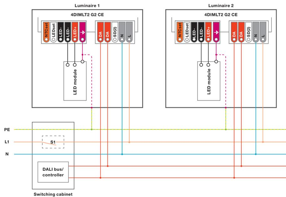
Up to 64 DALI LED drivers can be controlled via a two-wire control line – individually, jointly or in up to 16 groups. All of them are connected in parallel to the two DALI wires. DALI connections are not polarized. Therefore, plus and minus do not have to be checked. The maximum allowed wire length between two DALI LED drivers is 300 m. In case of problems, a DALI repeater has to be used.
