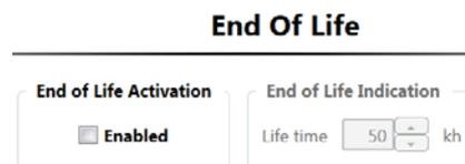
If the specified lifetime is reached, the LED driver indicates this through a lower light output during the first 10 minutes of the switch-on period as shown in figure 16.
