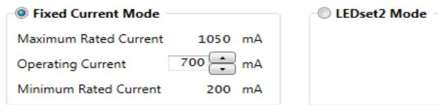
Without any resistor connected to the LEDset2 interface, the factory default current is 700 mA. As soon as the LED driver detects a resistor value for more than 3 seconds within the valid resistor range of 4.75 kΩ (1050 mA) and 24.9 kΩ (200 mA), it switches to the LEDset2 mode.
