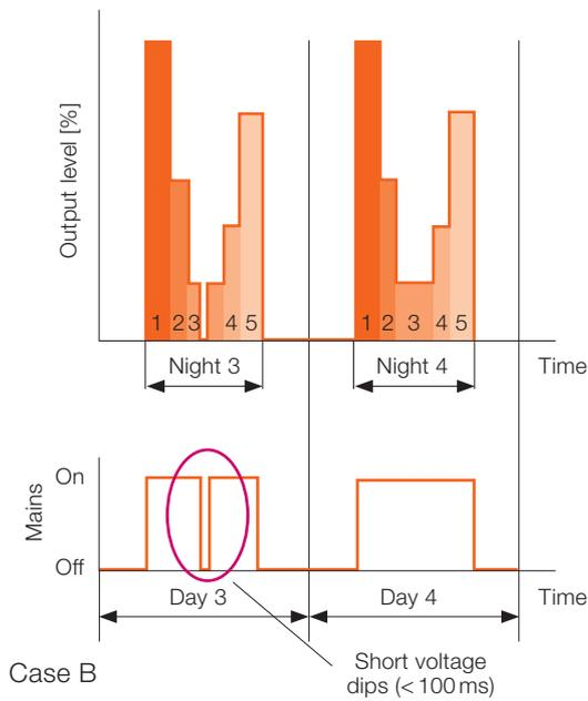
Voltage dips of less than 100 ms do not affect the on-time (case B).
