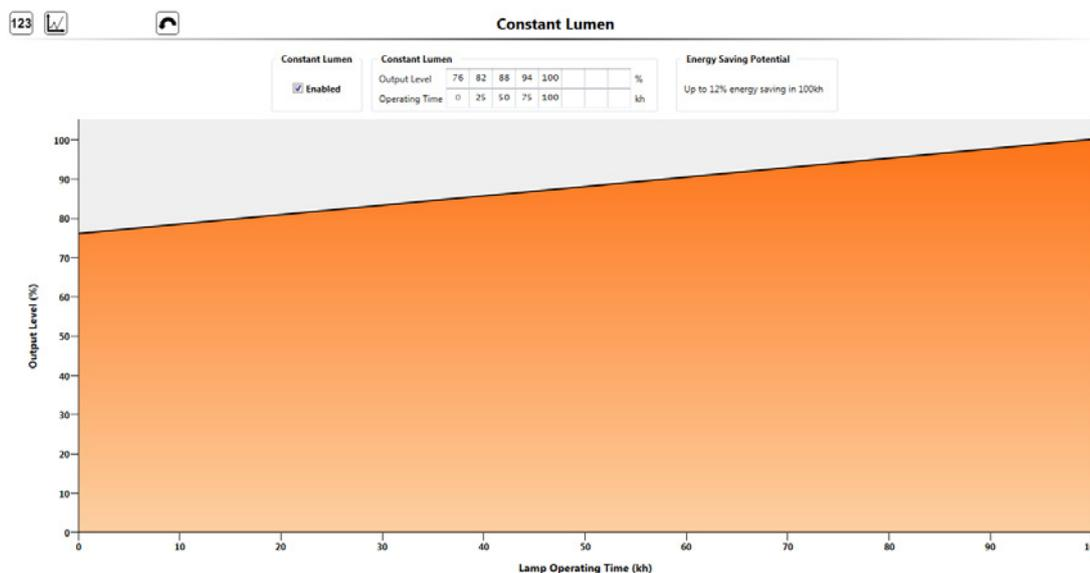
**Figure 16: “End of life” behavior without switch-on fade time**
