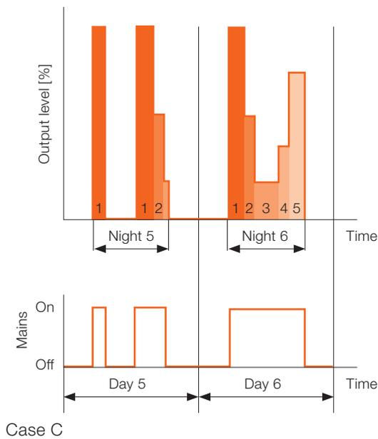
If the on-time of the LED driver is shorter than 4 hours, it is not saved and therefore not used to calculate the next on-time (case C).
