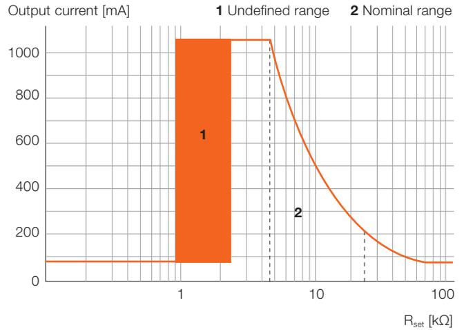
The corresponding output current can be calculated with the following formula within the valid resistor range ( $R_{set} = 4.75\text{--}24.9\text{ k}\Omega$ ):
