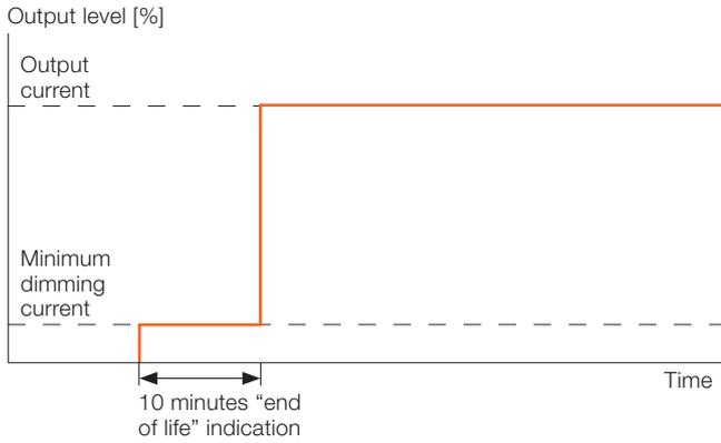
If a switch-on fade time is set, it is overridden by the “end of life” functionality as shown in figure 17. After 10 minutes, the output current is set according to the current switch-on fade time level.
