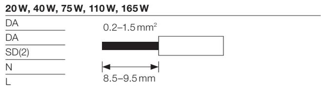
**Figure 43: Cable preparation, secondary side and equipotential pin**
