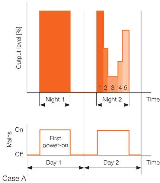
The AstroDIM profile is performed after the first valid on-time.
