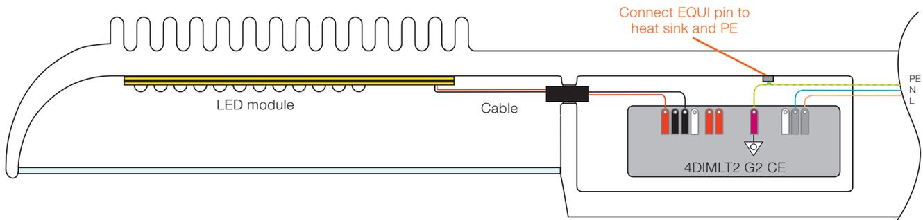
**Figure 45: Protection class II luminaire**
