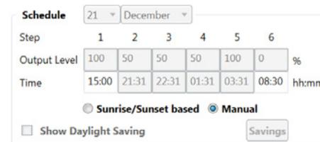
The AstroDIM function in astro-based mode relies on an intelligent algorithm. It starts after the first valid night and reaches its maximum precision after 8 valid days. A valid on-time is defined if the duration of the operation is longer than 4 hours and shorter than 24 hours.
