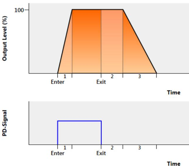
An active signal at the SD(2) port (PD signal) starts the presence detection profile, which is defined by the following four parameters:
