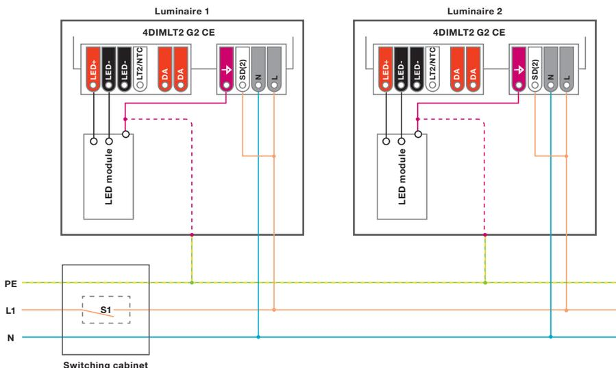
Figure 22: Wiring: AstroDIM (DALI) or AstroDIM PD (DALI)
