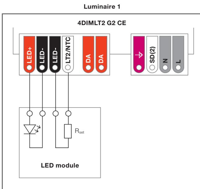
The LEDset2 coding for the 4DIMLT2 family is shown in the following graph.
