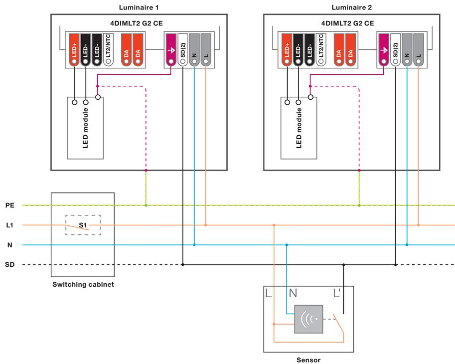
Figure 28: Presence detection in AstroDIM mode
