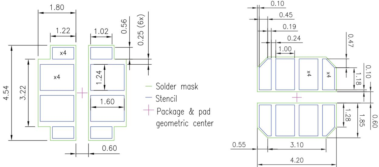
Figure 3a. Recommended PCB footprint showing solder mask and stencil opening for LUXEON 5050 (Round LES), left, and LUXEON 5050 (Square LES), right. Dimensions are in mm.
