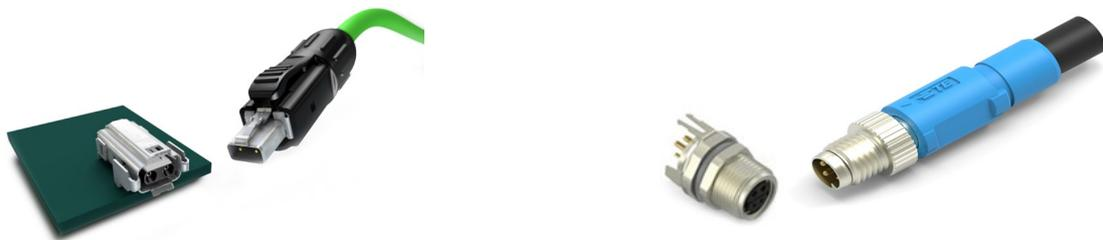
Figure 1: Single Pair Ethernet connectors per IEC 63171-6: (a) IP20 connector for SPE where power may be delivered via PoDL with max. 1,36 A (b) IP67 hybrid connector for SPE with separate power contacts allowing for currents up to 8 A
