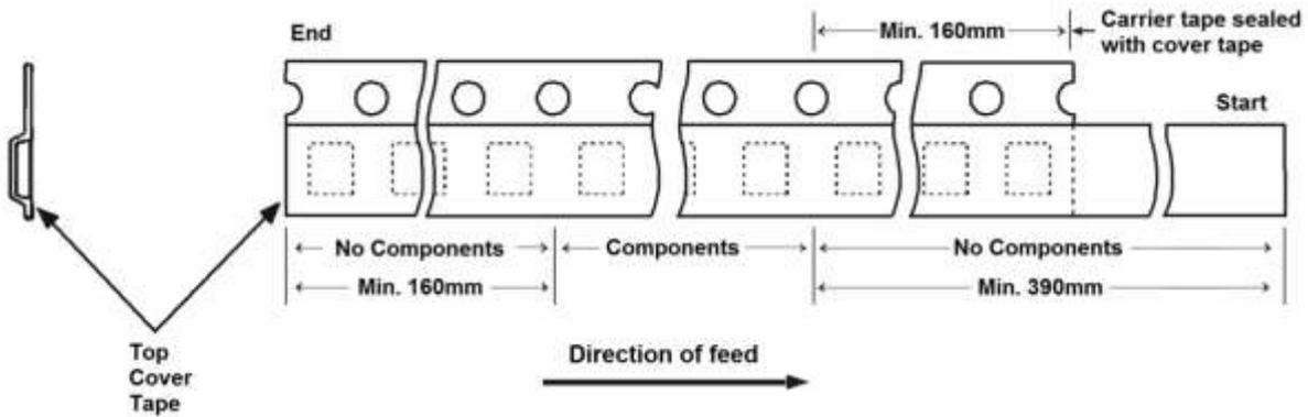
**Note:** There shall be a leader of at least 230mm which may consist of carrier tape and/or cover tape or a start tape followed by at least 160mm of empty carrier tape sealed with cover tape.
