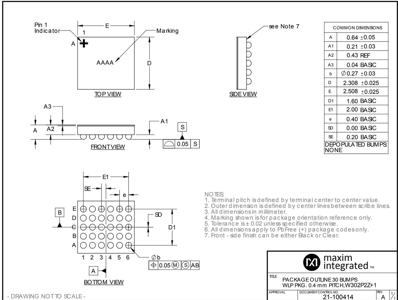
For the latest package outline information and land patterns (footprints), go to [www.maximintegrated.com/packages](http://www.maximintegrated.com/packages). Note that a "+", "#", or "-" in the package code indicates RoHS status only. Package drawings may show a different suffix character, but the drawing pertains to the package regardless of RoHS status.
