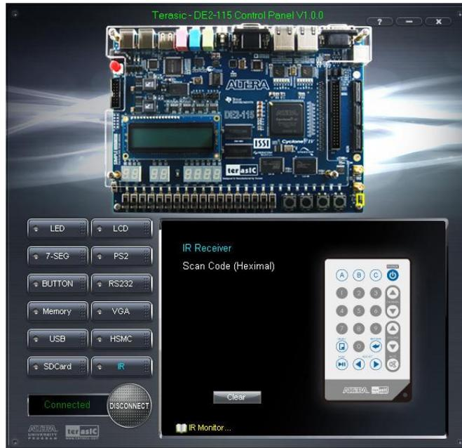
Figure 3-14 Testing the IR receiver using remote controller
