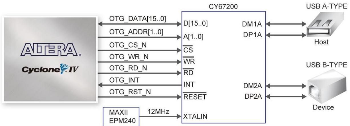
Figure 4-31 Connections between FPGA and USB (CY7C67200)
