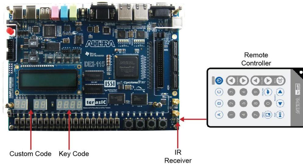
Figure 6-22 The Setup of the IR receiver demonstration
