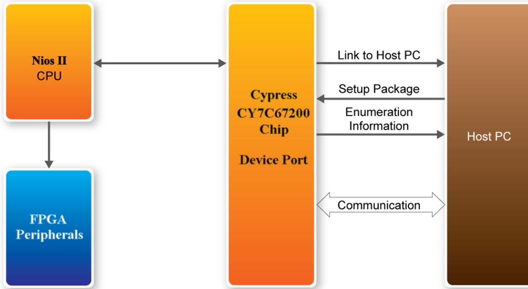
Figure 6-5 Block diagram of the USB device demonstration
