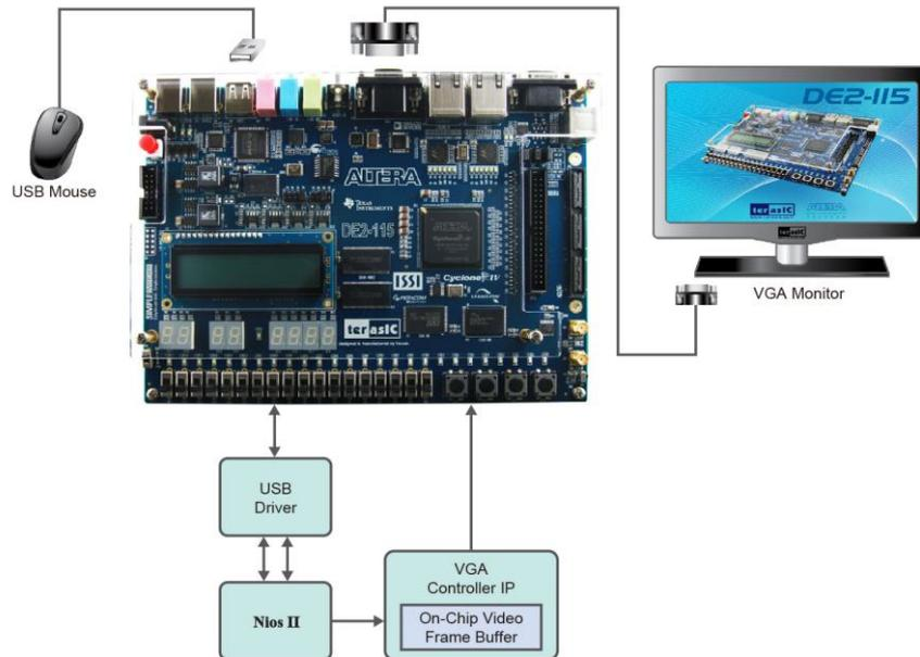
Figure 6-4 The setup for the USB paintbrush demonstration
