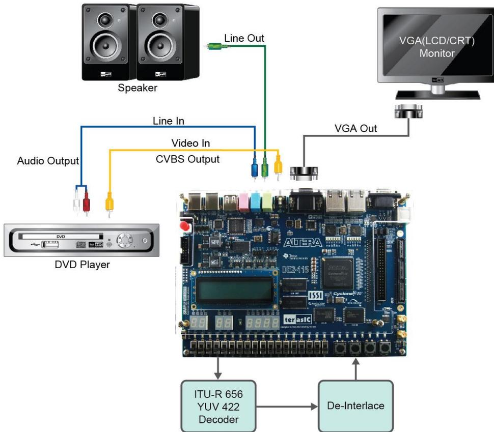
Figure 6-2 The setup for the TV box demonstration
