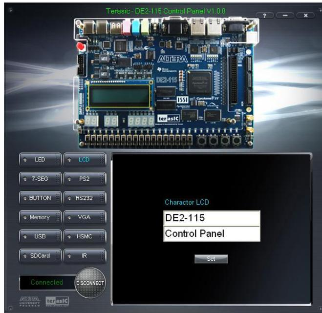
**Figure 3-5 Controlling the LCD display**
