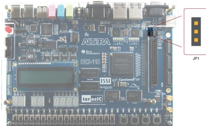
Figure 4-28 Working mode setup header for Ethernet PHY
