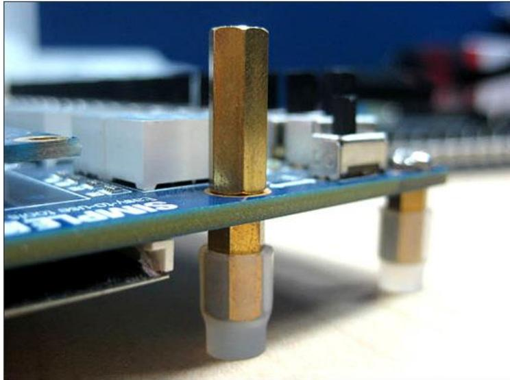
**Figure 1-2** The feet for the DE2-115 board
