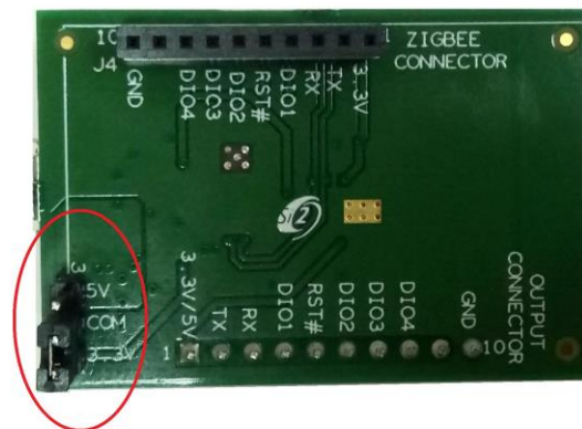
Figure 11: Showing Shorting Jumper placement 3.3V selection
