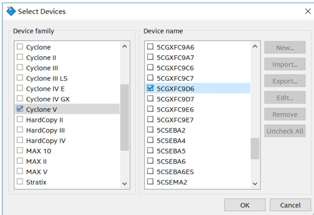
**Figure 6-5 Select Devices page for GX device**
