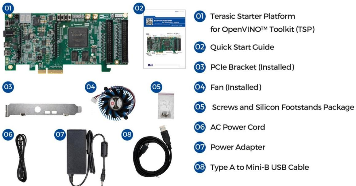
**Figure 1-1 Starter Platform for OpenVINO™ Toolkit package contents**
