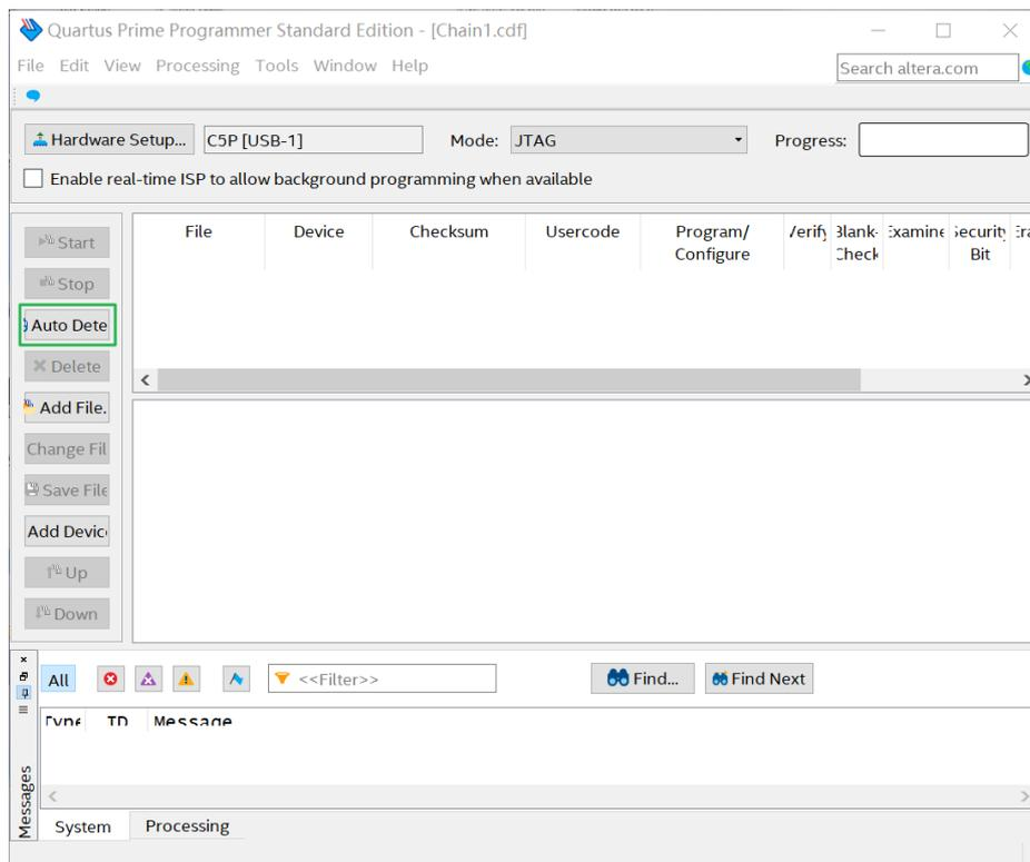
**Figure 3-2 Detect FPGA device in JTAG mode**
