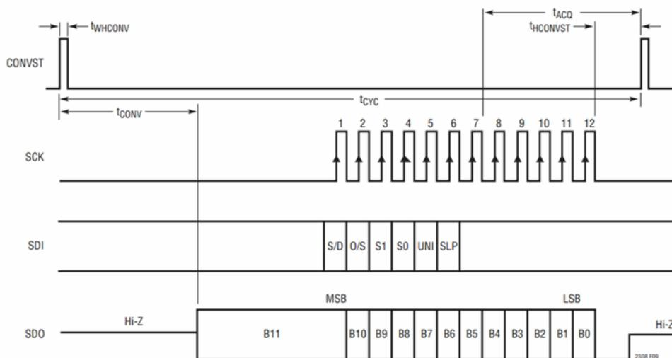
**Figure 5-18 LTC2308 Timing with a Short CONVST Pulse**
