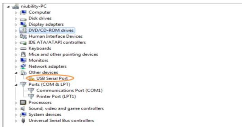
**Figure 5-9 Unrecognized USB Serial Port on PC**
