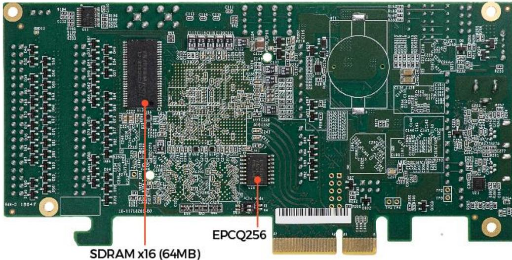
**Figure 2-2 Starter Platform for OpenVINO™ Toolkit (bottom view)**
