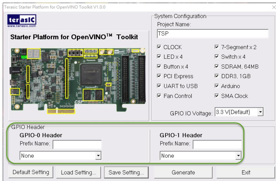
**Figure 4-5 GPIO Expansion**
