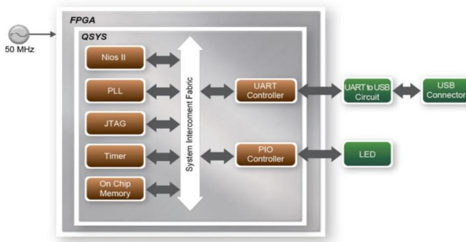
Figure 5-8 Block diagram of UART Control LED demonstration
