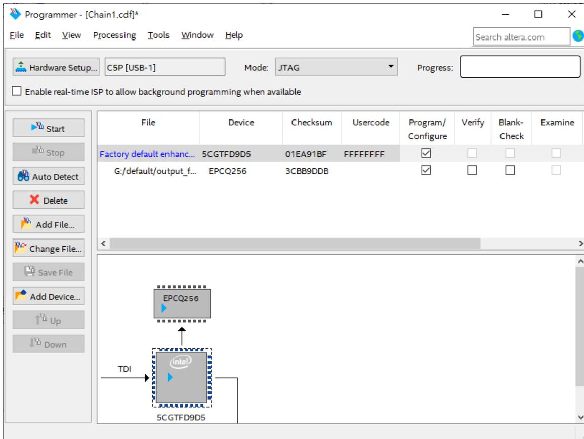
**Figure 6-8 Quartus Prime Programmer window with .jic file**
