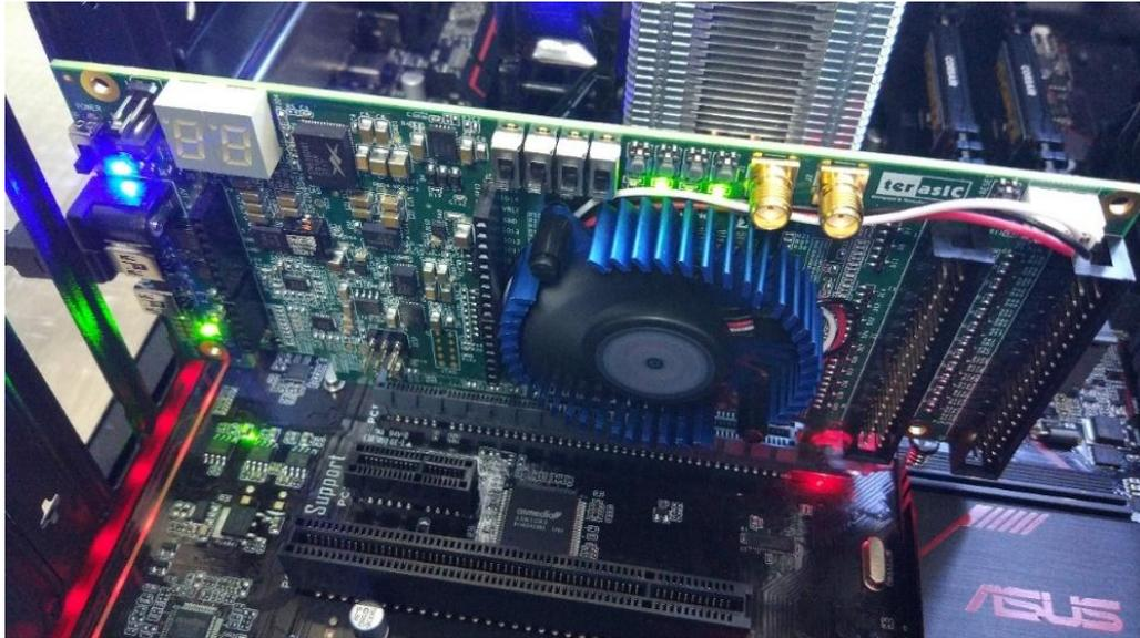
**Figure 7-3 Install the FPGA board on the PC**
