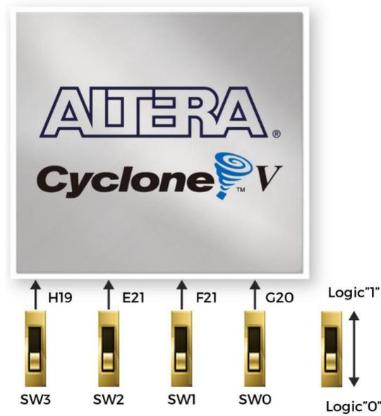
**Figure 3-15 Connections between the slide switches and Cyclone V FPGA**
