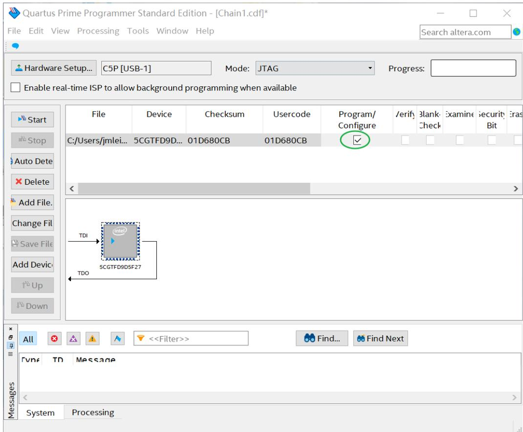
**Figure 3-9 Program .sof file into the FPGA device**
