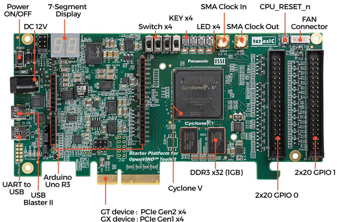
Figure 2-1 Starter Platform for OpenVINO™ Toolkit (top view)
