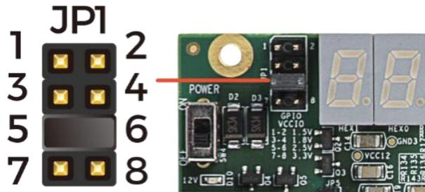
**Figure 3-23 Short pin5 and pin 6 of JP1**
