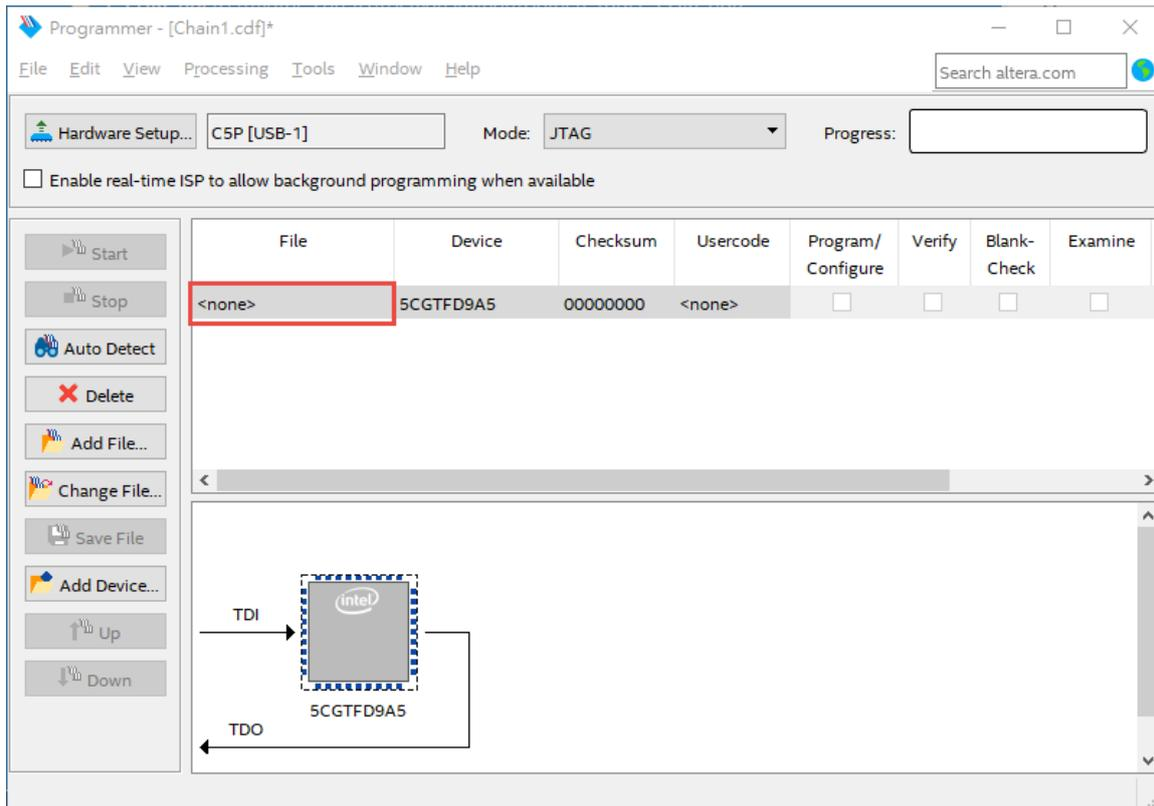
**Figure 6-7 Quartus Prime Programmer detects the FPGA device**
