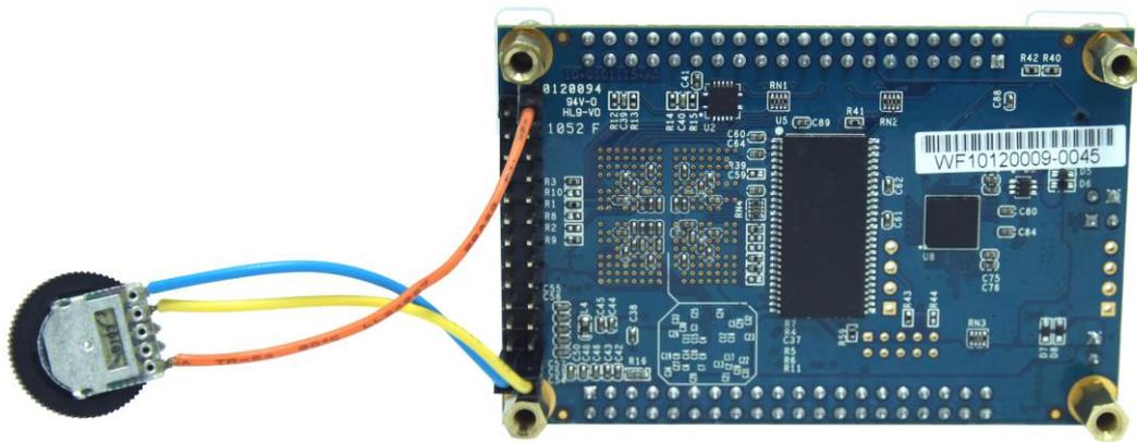
Figure 8-5 ADC Reading hardware setup
