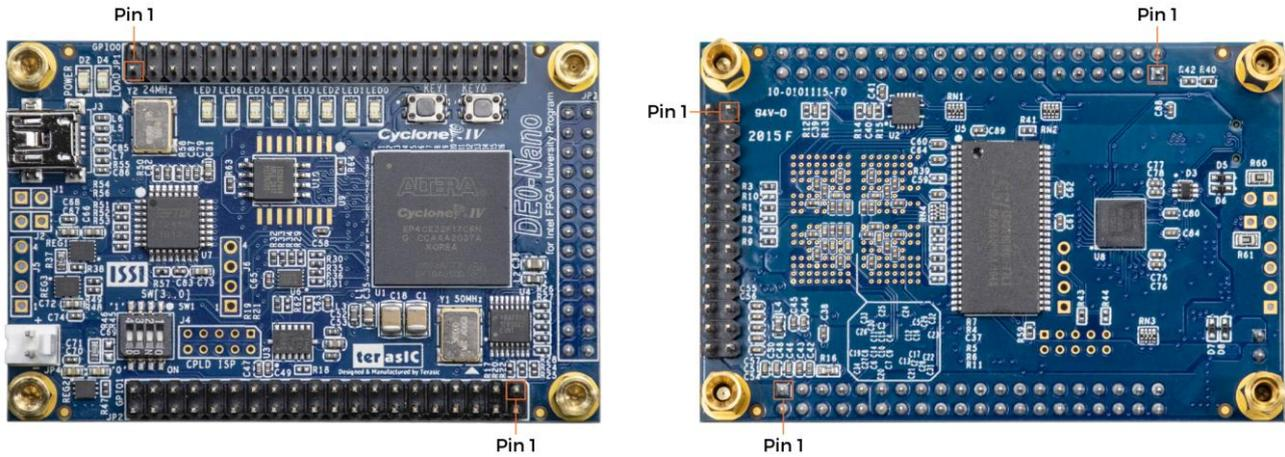
Figure 3-12 Pin1 locations of the 2x13 header
