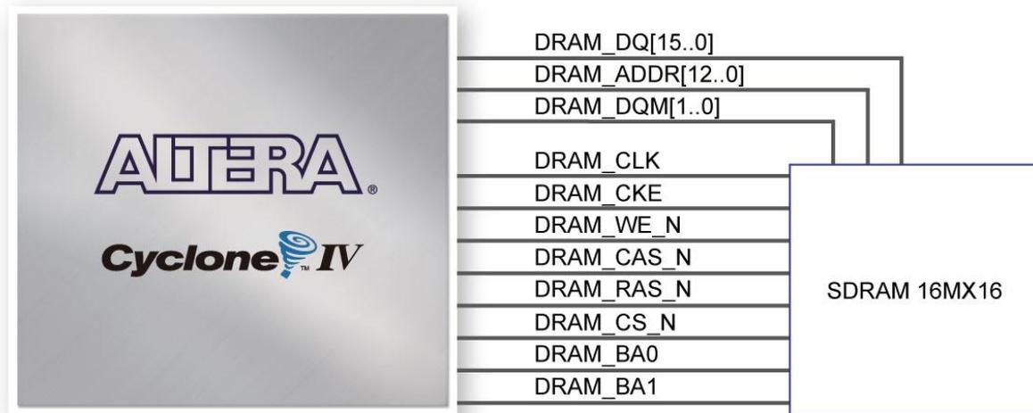
**Figure 3-6 Connections between FPGA and SDRAM**
