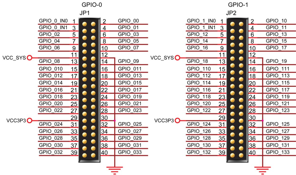
Figure 3-8 Pin arrangement of the GPIO expansion headers
