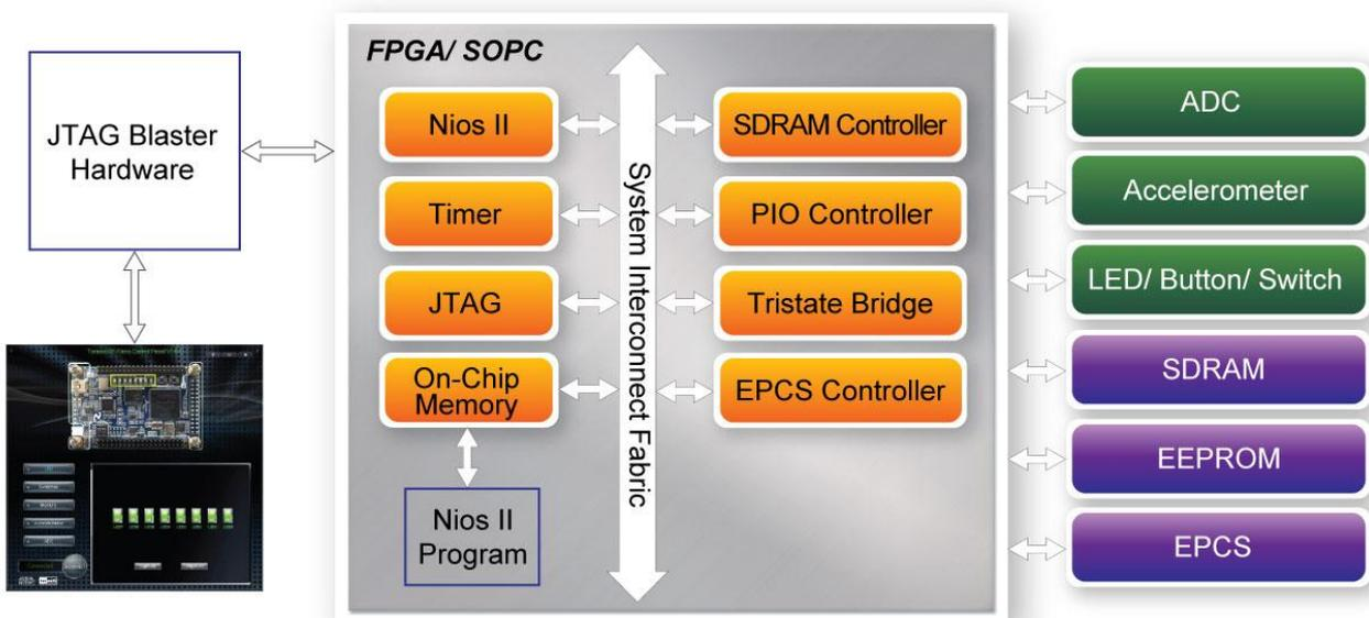
Figure 4-8 The block diagram of the DE0-Nano Control Panel
