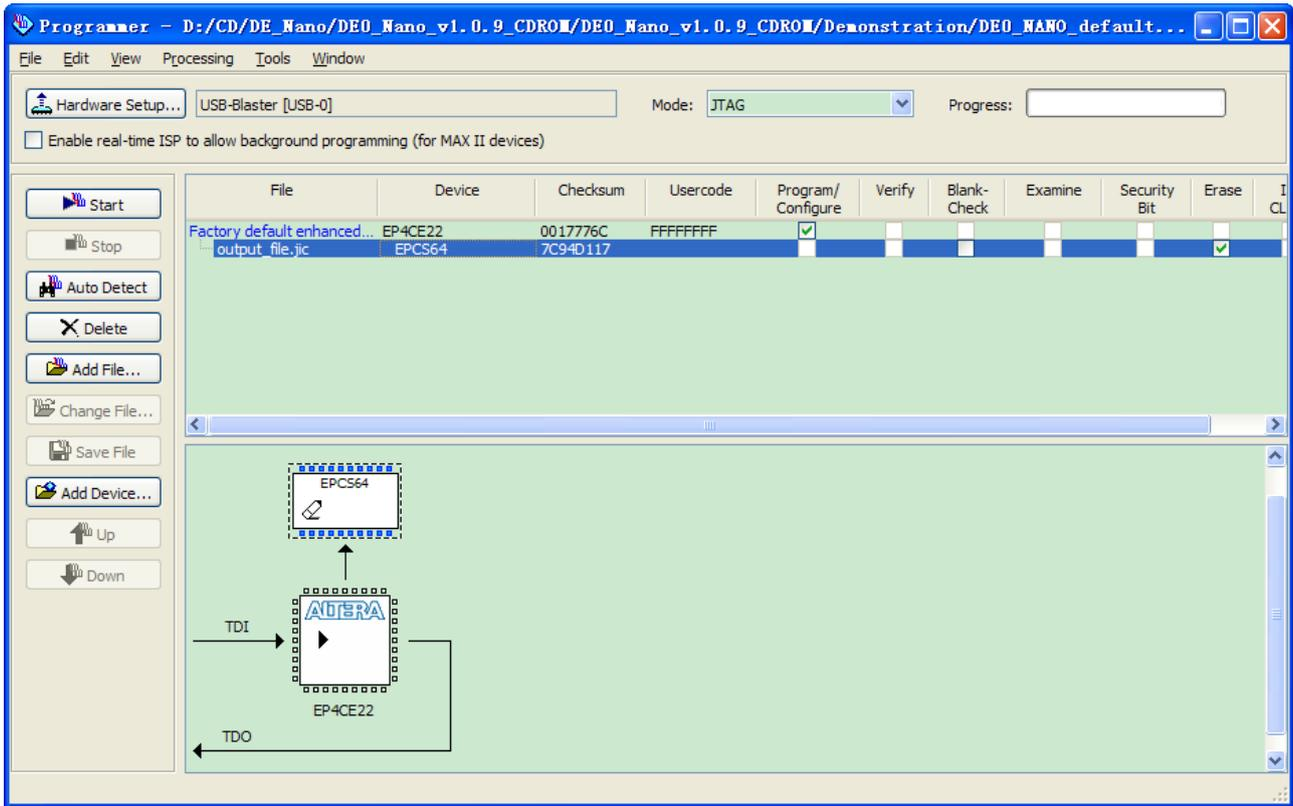
**Figure 9-7 Erasing setting in Quartus II programmer window**
