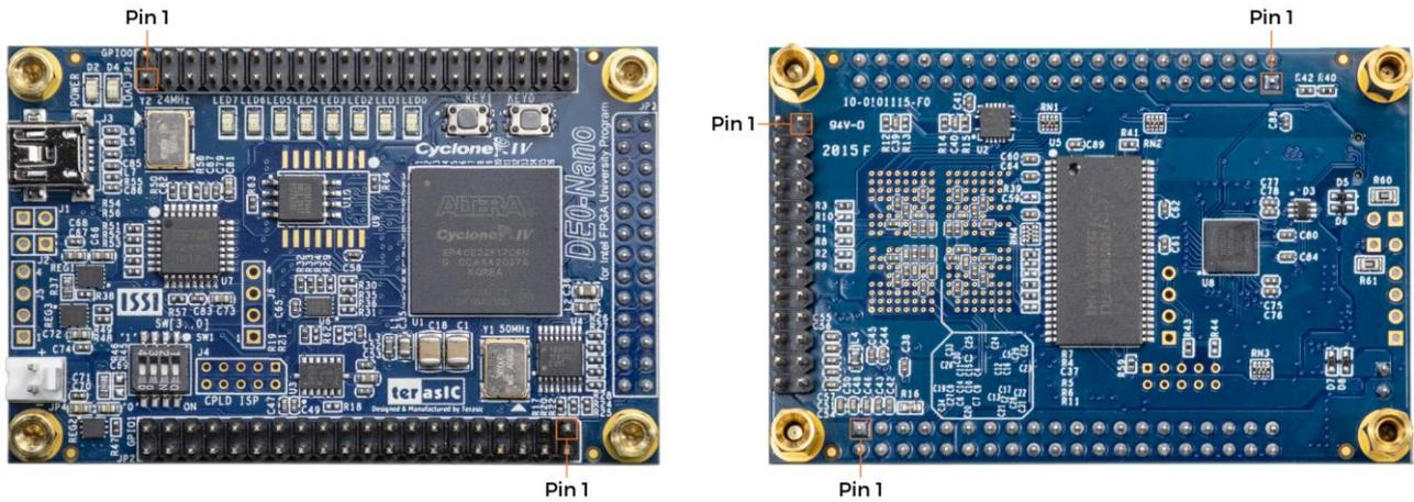
Figure 3-9 Pin1 locations of the GPIO expansion headers
