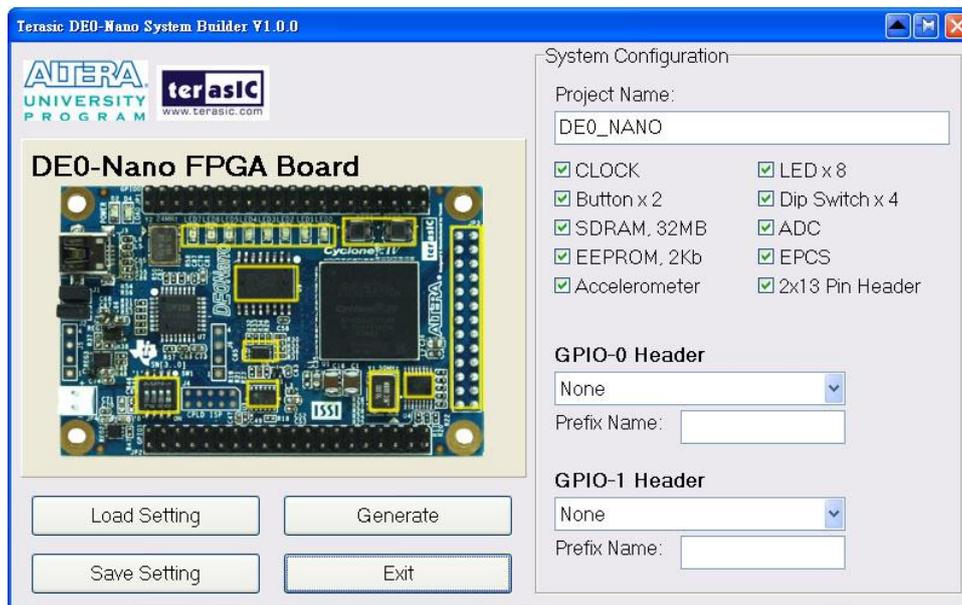
**Figure 5-2 The DE0-Nano System Builder window**
